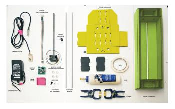
Figure 4: All the parts needed for one cardboard mMTM stage.
