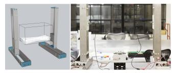
**Figure 2:** A 5-axis (4-axis wire control, 1 rotary table) hot-wire cutter made with the m[MTM] machine parts.
