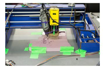
Figure 5: Workshop participants test the mechanical limits of the cardboard plotter they have just developed by turning it into a CNC mill.
