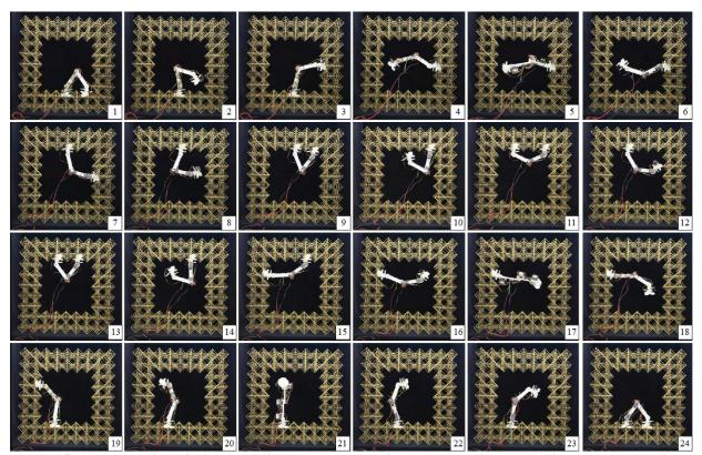
**Figure 15: Demonstration of climbing 360° around a loop using ankle rotation and upside down locomotion.** In steps 1-7, the robot uses ankle rotation to climb to the upper surface of the structure. In steps 8-13, the robot steps along the upper surface of the structure while hanging upside down. In steps 14-24, the robot uses two ankle rotation maneuvers to step to the side of the structure and then to return to its original position. Total elapsed time: 10 min.
