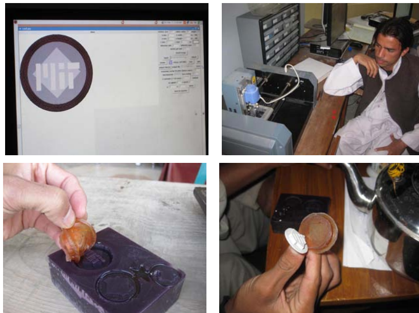
Figure 17: Custom coins or medals are cast from urethane molds. In this process, users create a 3D image in a block of wax using the precise 3-axis computer controlled mill. A negative urethane mold is made from the wax coin. The mold can be used repeatedly without a releasing agent to make copies of the coin in a variety of materials.
