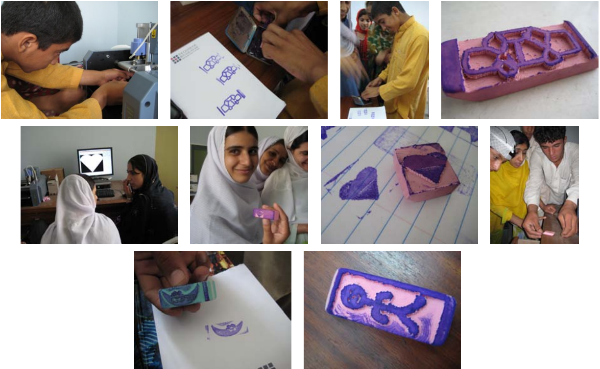
Figure 16: Making custom stamps by machining rubber erasers with a 3-axis mill is a fast, safe, and rewarding way to learn 3D design.
