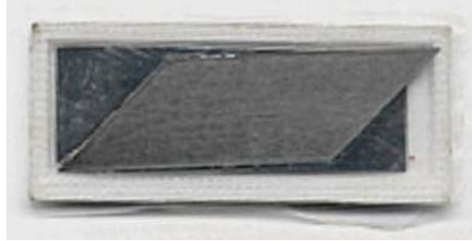
Figure 16. Electronic Article Surveillance label (Ultramax™ label by Sensormatic, Inc.) containing magnetoelastic strip and trapezoidal bias magnet.
