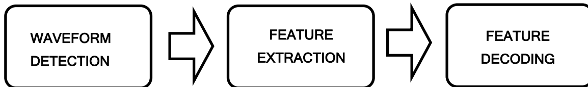
Figure 11. Data decoding process employed by a chipless reader.
