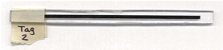
Figure 55. Photograph of amorphous ribbon material used for study.
