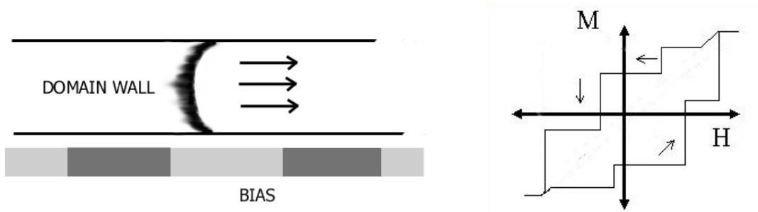
Figure 53. Schematic illustrating domain wall motion in the presence of a non-uniform magnetic field bias (left); idealized M vs H loop for this structure (right).
