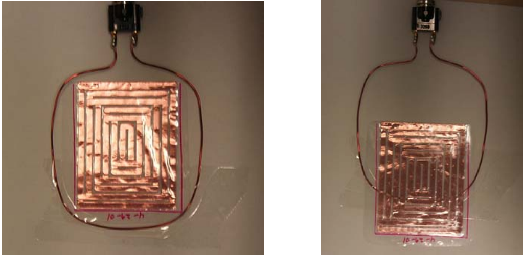
Figure 87. Photograph of loop antenna used as test probe. The photo on the left shows the standard measurement geometry. The photograph on the right depicts a misaligned tag which gives rise to additional parasitic resonances.
