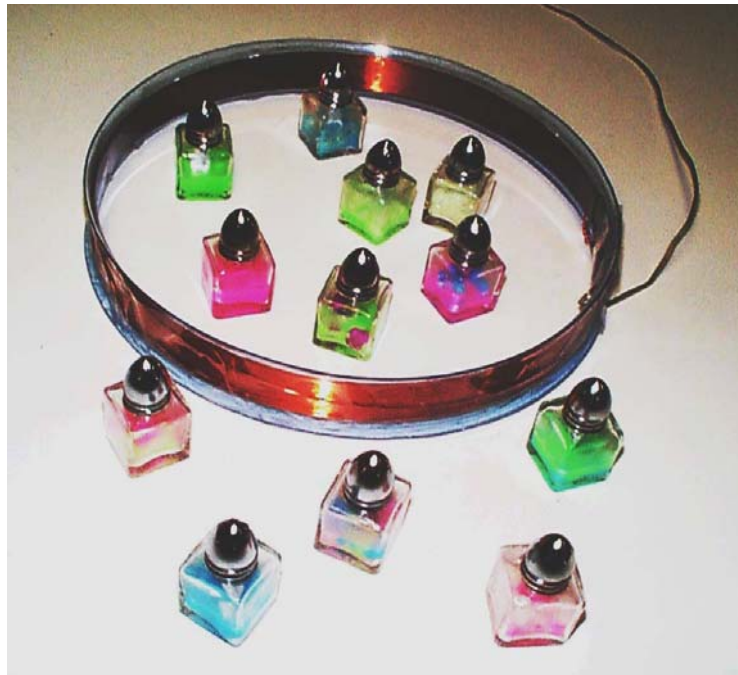
Figure 63. Portions of an October 1997 demonstration employing one dozen distinguishable items tagged with magnetoelastic resonators.
