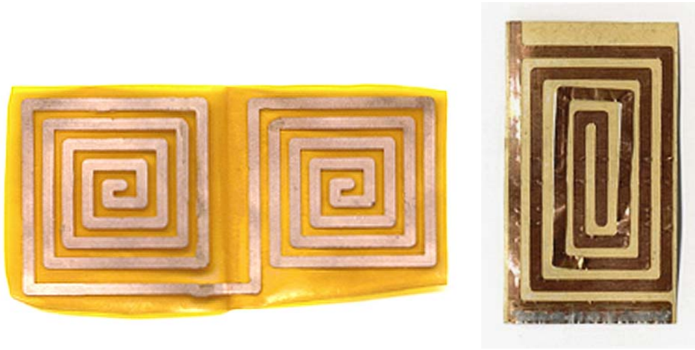
Figure 69. Photograph of two different tag designs employing distributed capacitance. The tag on the left is shown unfolded and the photograph on the right shows a single layer of a tag.
