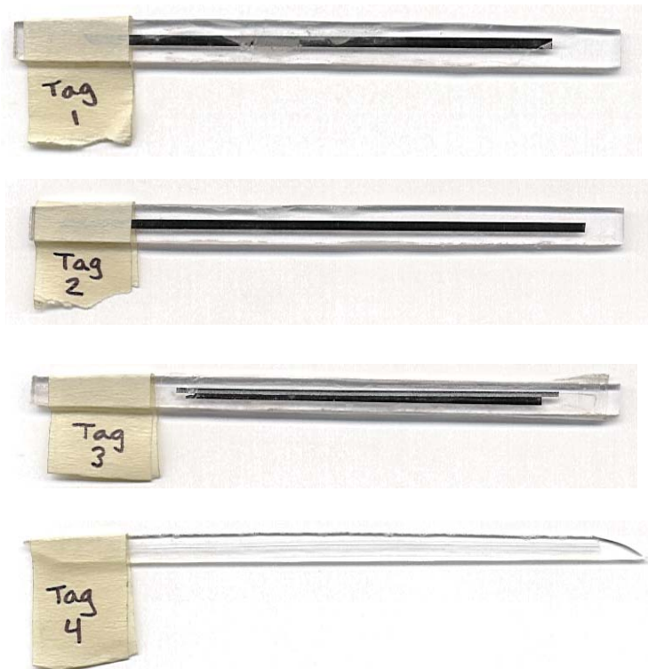
Figure 58. Photograph of VCB magnetic strips mounted on Plexiglas employed for the time-domain measurements. The strip on the bottom (#4) is an amorphous wire sample made by Unitika in Japan.
