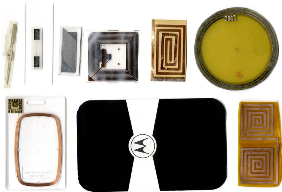
Figure 118. Photograph of a variety of electromagnetic tags, photographed to scale, including both EAS and RFID labels.
