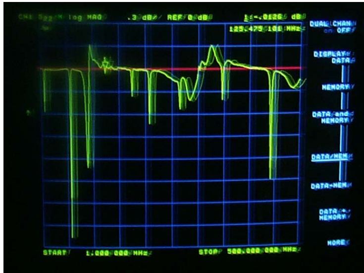
Figure 89. Frequency spectra from misaligned tag, showing additional resonances arising from non-uniform field excitation.
