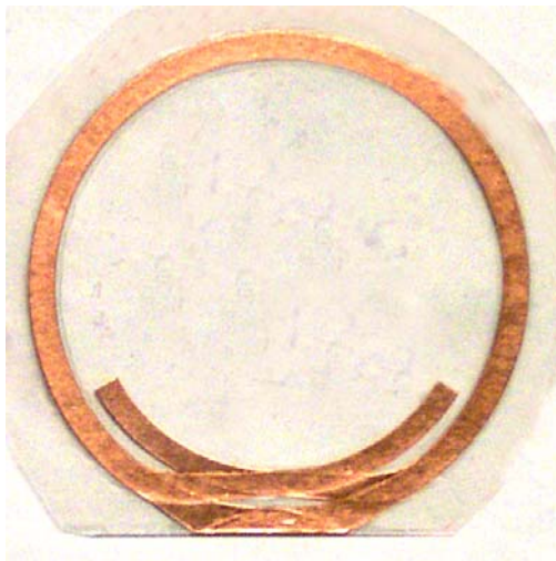
Figure 93. Photograph of sample single resonance tag used in the parameter study. The tag shown has \Theta = 420^\circ with diameter = 2.5 inches.
