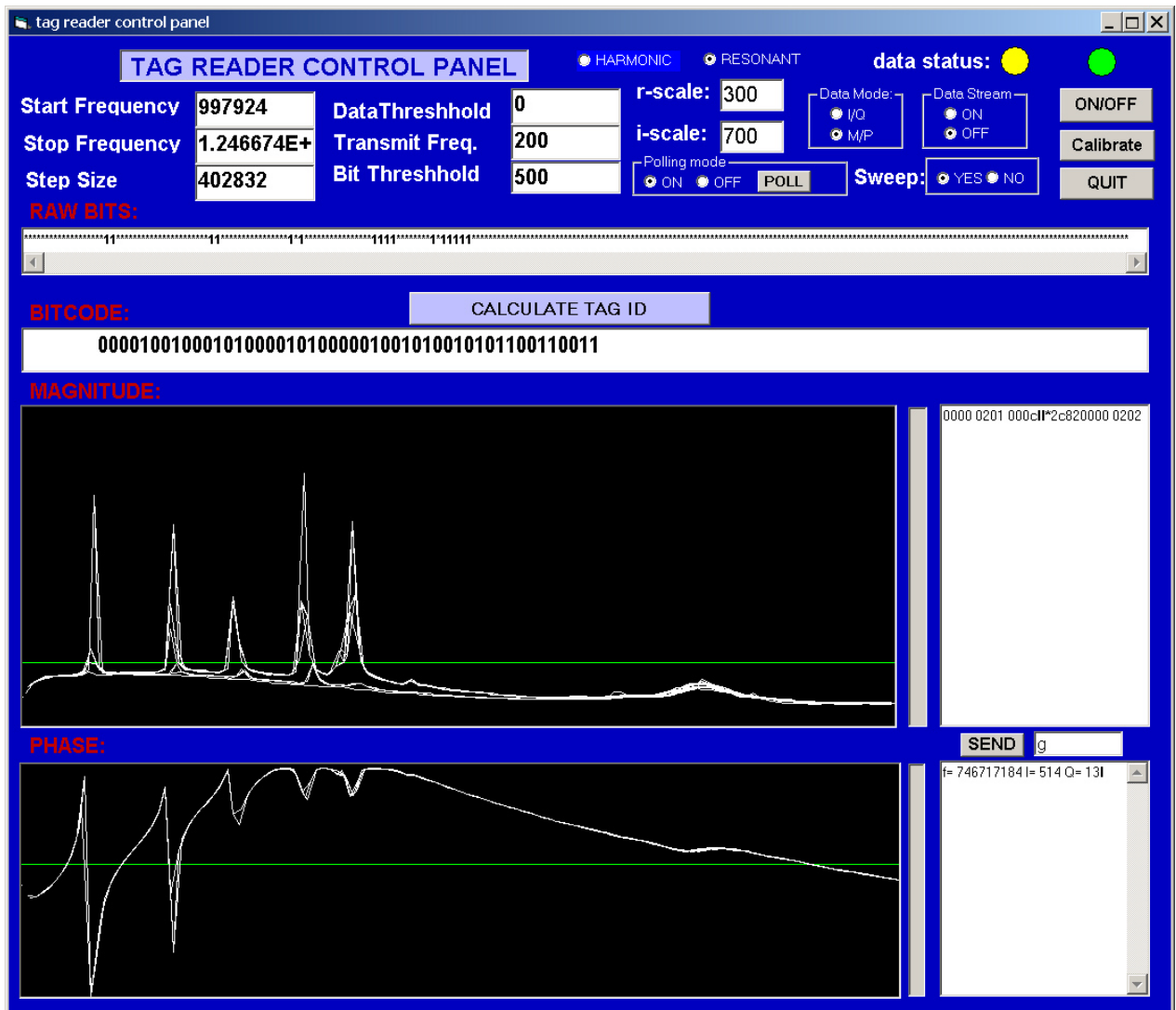
Figure 105. PC Windows interface implemented in Visual Basic showing spectra for a multi-resonant tags and also displaying the raw frequency bin data bits as well as a compact “bitcode” representation
