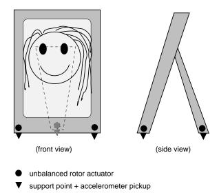
Figure 2.5. Schematic view of the Inertial Frame interpersonal haptic communication device.
