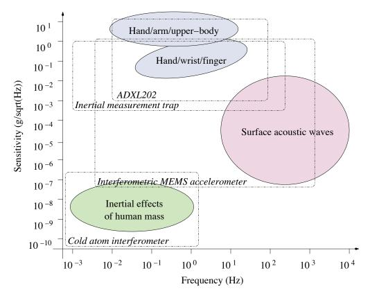
Figure 2.2. Inertial UI signals and sensor capabilities.
