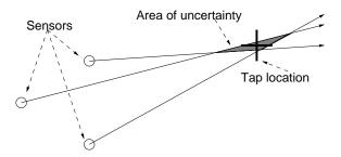
Figure 2.6. Tap location using multiple orientations.
