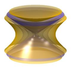
**Figure 3.2.** Isopotential surfaces of  $\Phi \propto (r^2 - 2z^2)$ .
