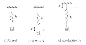
Figure 3.1. Spring-mass accelerometer.
