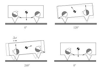
Figure 2.4. One "hop" cycle using unbalanced rotors dephased by 120°, resulting in a net displacement  $\Delta x$ .
