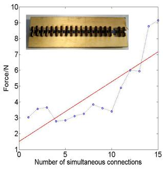
Figure 6: The force necessary to simultaneously separate a number of GIK bricks as a function of the number of GIK bricks that need to be separated.
