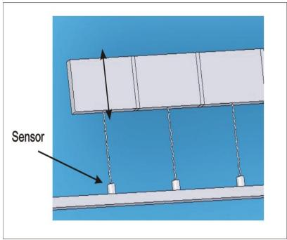
Figure 24: The error detection blade is composed of a touch pad which is able to move up and down and a sensor which is sensing how much pressure is applied against each touch pad. An error is detected if there is a too high pressure difference between 2 adjacent pads.
