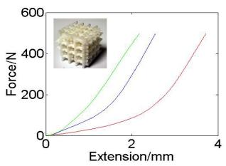
Figure 9: Isotropy tunability: different Young moduli in different directions.
