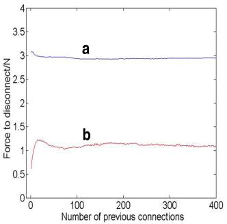
Figure 5: The variation of the force necessary to disconnect 2 GIK bricks as you connect and disconnect the 2 same bricks
