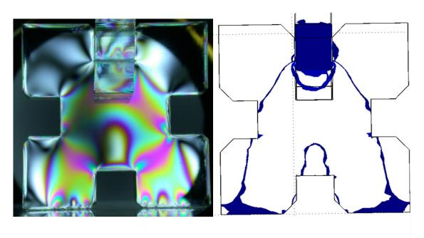
Figure 4: The measured (left) and calculated (right) stress pattern in a GIK brick loaded on the top.
