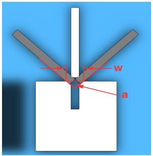
Figure 7: Drawing explaining how error tolerance can allow 2 GIK bricks to connect even if they aren't perfectly aligned.
