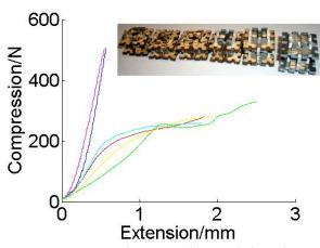
Figure 10: Mixed material tuneability: by varying the ratios of plywood and aluminum the Young modulus is varied.
