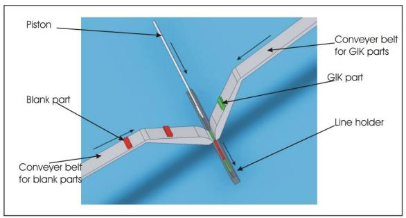
Figure 25: Scheme of a feeder formed by 2 conveyor belts, one for vertical GIK one for Blanks. If more than 2 parts are needed more conveyor belts can be added. The parts are deposited in a line holder (dark gray) and a piston pushed the parts in the head when the line is built.
