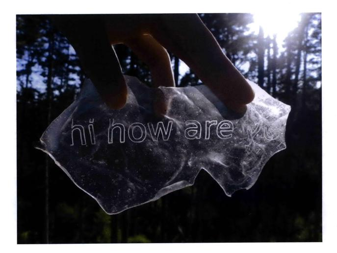
Figure 7.15: A laser etched sheet of potato starch film. The potato film was dried outside, which caused the imperfections on the film you see here. Potato starch film can easily be laser etched or cut, although even so the applications remain limited.
