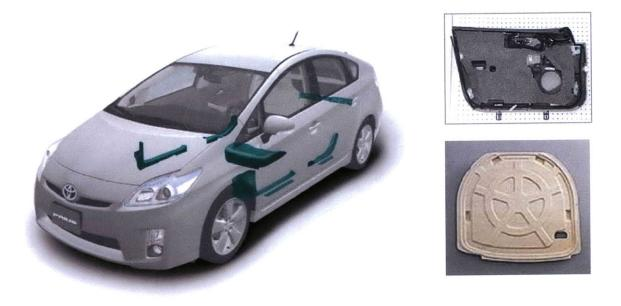
**Figure 4.4:** In the Toyota Prius, several interior components are now made with kenaf/ramie reinforced PLA. On the right the parts of the interior that are made with green composite are shown in green. On the left is a side door cover and a spare tire cover made with kenaf reinforced polypropylene. Images from toyota.co.jp.
