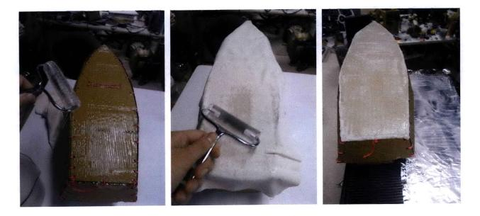
Figure 7.8: Using wet corn starch paste for linen and cornstarch lay-up. The resulting composite is stiff but very sensitive to moisture. Between each ply the composite must be set to dry completely,
