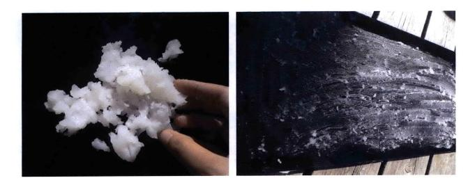
**Figure 7.6:** The corn starch paste can be spread either while hot or after it has cooled. If the paste is spread hot, it will shrink considerably while drying. This is a difficulty with making large sheets. If the corn paste is too cool, it will have already set, and it will not spread into a thin film like you can see in the photo on the right.
