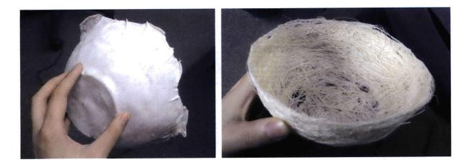
**Figure 7.10:** Jean-Baptiste Labrune used boiled corn starch, rayon (left) and sisal (right) to make bowl shapes. Even with only one ply of jersey-knit rayon, he was able to keep the form of the mould. The jersey-knit fabric allows the fibre to conform better to the shape of the mould.
