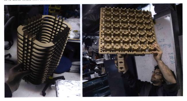
Figure 7.1: Using 2D tools to make 3D jigs for fibre lay-up methods. On the left a laser-cut press-fit cardboard mould which was later coated in a rayon-epoxy composite. On the right Jonathan Ward's digital assembly kit, made of pieces of plywood cut on a ShopBot CNC mill. See also [51].
