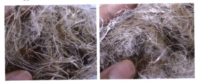
Figure 3.4: Left: Raw hemp fibres from Hemp Traders ltd. in Santa Monica, CA, Right: Washed kenaf fibres, FK100 DSAT 50mm fibres from Bast Fibres LLC New Jersey.
