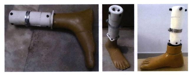
**Figure 7.32:** Extension pylon attached to two different paediatric Jaipur feet. The first has a very high ankle block, and the pyramid that is attached to it is too large for ankle. The second has a locally manufactured cast metal pyramid, but that pyramid is only screwed in in the centre, causing rotational play.
