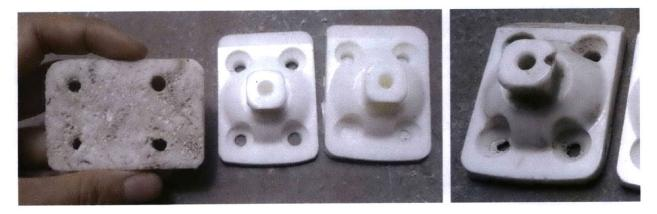
**Figure 7.26:** Casting a standard sized pyramid of Smooth-cast 300 polyurethane with kenaf reinforcements, Smooth-cast 300 polyurethane only, and Task 4 polyurethane. All casting resins from Smooth-on. On the right the top view of the kenaf-reinforced polyurethane.
