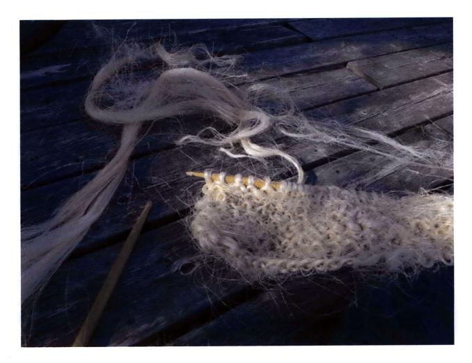
**Figure 7.16:** Because of the lack of woven or knit structural natural fibres (like sisal, which in strength is comparable to fibreglass), this was an exercise in getting long sisal fibres into a sheet. The hand-knitted sisal unfortunately did not have uniform stretching properties. However, if knit with more care, knit natural fibres could be useful in making sheets that can attain non-zero Gaussian curvature during composite lay-up.
