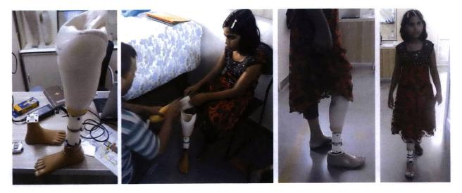
**Figure 7.34:** Patient testing the extension prostheses. The Jaipur foot is only available with a relatively high ankle block (see feet on left), leaving little room for the pylon and its extension. Finally we tested the extension pylon with a low-profile SACH foot (right).
