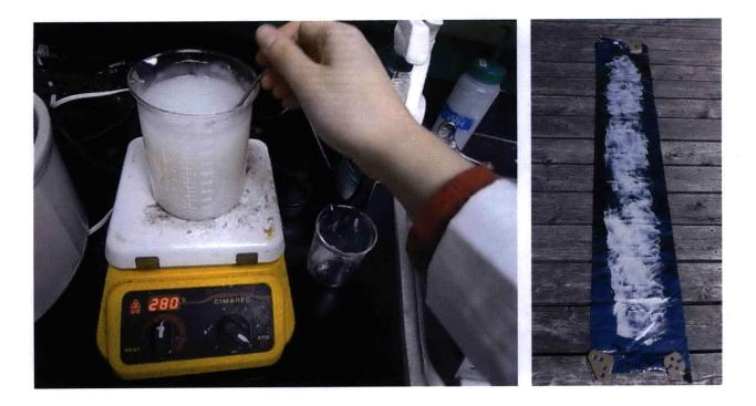
Figure 7.5: Plasticising corn starch with glycerol, alcohol, white vinegar and water and sun-drying the resulting paste on aluminium foil. Sun drying is faster, but can lead to more cracking and also exposes the film to dust and particles from the outdoors.
