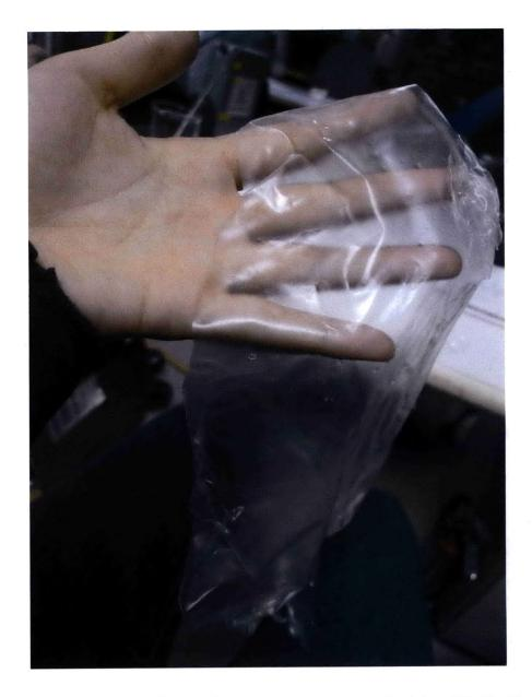
**Figure 7.7:** A sheet of corn starch film, dried at room temperature on aluminium foil. The film after curing is sensitive to ambient moisture, and can shrivel or crumple if stored with uneven amounts of humidity on either side of the sheet. The tensile strength and elongation at break is highly dependent on the plasticisers used and their ratios.
