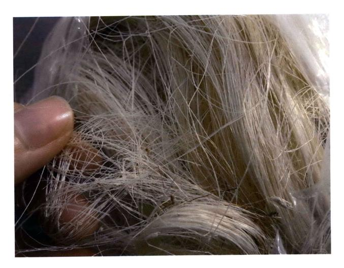
**Figure 3.2:** Decorticated sisal fibres from Reynolds Advanced Materials, Boston MA. Even within a single sisal fibre (which is a bundle of elementary fibres) there is a variation in width of up to 200%. The different part of the leaves produce different qualities of fibre, and this must be taken into account when producing parts with sisal.
