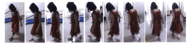
**Figure 7.36:** The foot used in this test prosthesis is too large for the patient, making her gait poor during testing. She is unsure of her toe-off, and so looks at her feet as she is walking. The pylon makes some noises as some parts with play rub against each other, making her further uncertain of the prototype. As time went on, she became more comfortable, but still had awkward gait due to the wrongly sized foot.
