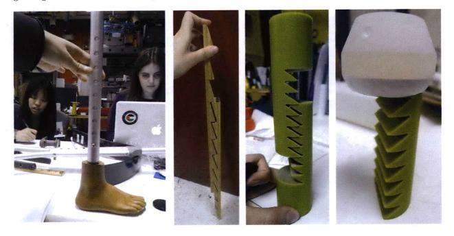
**Figure 7.23:** Several design iterations for the extension pylon. In the left most photo (a) Cindy Oh on the left, Deema Totah on the right with a recycled aluminium crutch on a Jaipur foot. (b) A stepping design for extension, prototyped out of wood on a bandsaw. (c) A nylon rod cut to be extendable on the waterjet cutter (d) Nylon extension fitted with a 3D printed female pyramid, ready to be used to make a mould.
