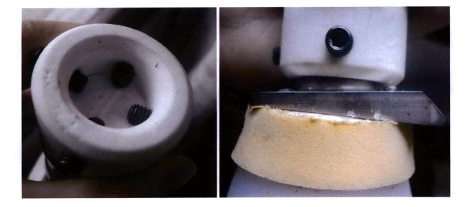
**Figure 7.30:** The female part of the pyramid does not have to have the same material strength. As long as the material retains the set screws without slippage and does not crack under normal load, it is strong enough for the female adaptor. On the right the hemp-epoxy flattened socket with a machined titanium male pyramid and a polyurethane female pyramid.
