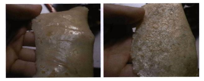
Figure 7.2: Using soy protein isolate obtained from Barry Food Farms inc., glycerol and deionized water, I made some protein sheets like described in [26]. These first few attempts had trouble with uniform curing, and would result in flakey tops or gel-like bottoms that would later crack.
