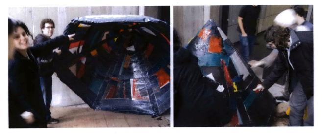
Figure 7.9: David Robert, David Cranor and Edwina Portocarrero built an inflatable mould which they used to lay up recycled apparel fabric with epoxy resin.
