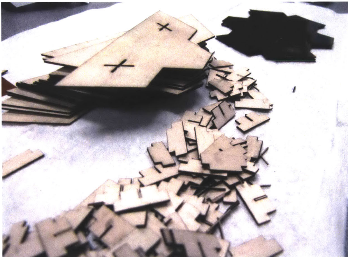
Figure 6.4 Joint inserts and rigid components for the outermost layer of the pressure vessel prototype
