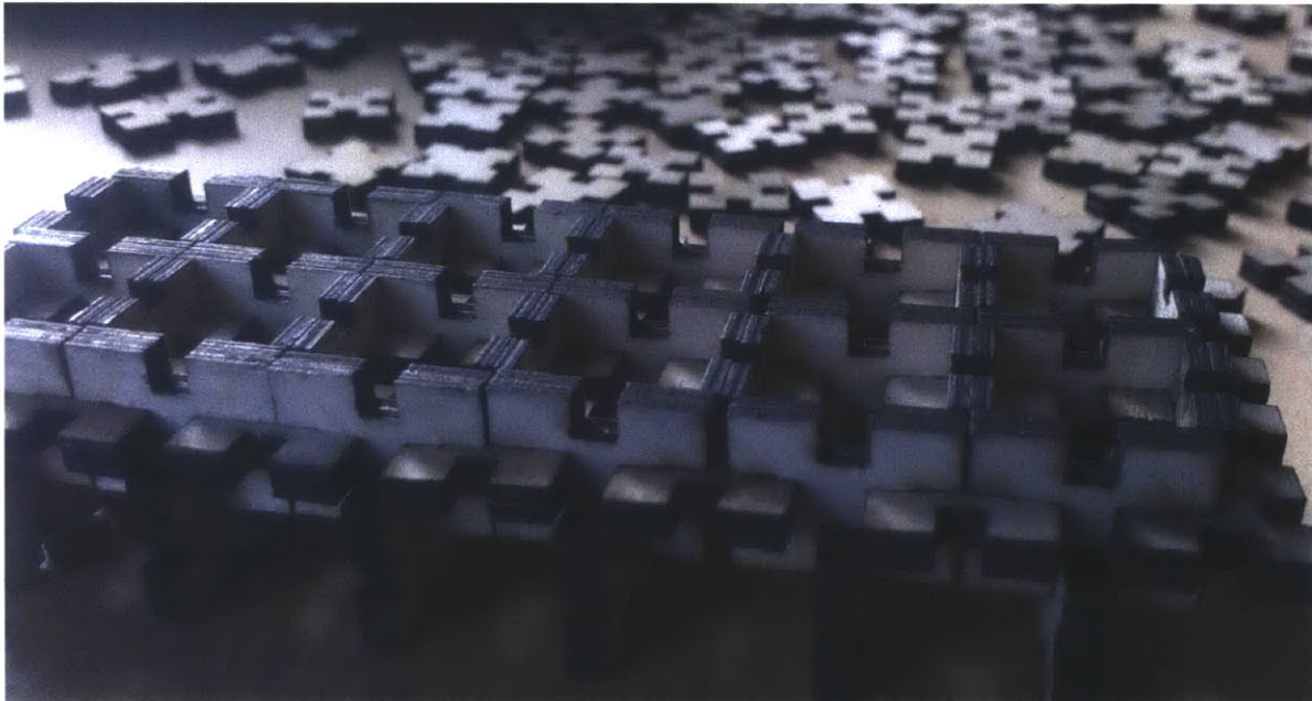
Figure 3.3 Press Fit GIK components laser cut and assembled by hand
