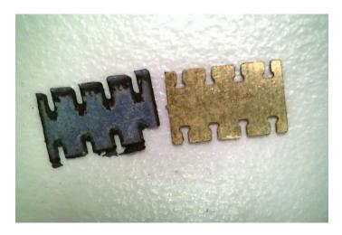
Figure 2-12: Excimer cut part next to brass part produced using the Wire-EDM.
