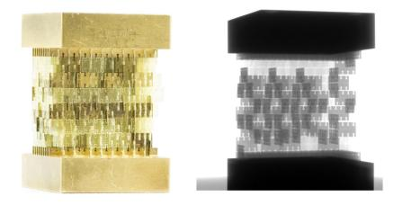
Figure 4-6: A discretely assembled inductor with an x-ray view of the interior.
