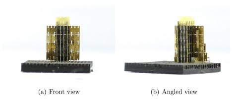
Figure 4-7: A discrete resistor assembled from anti-static polymer parts.
