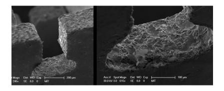
Figure 7-18: SEM micrograph of a slot that has not been used.
