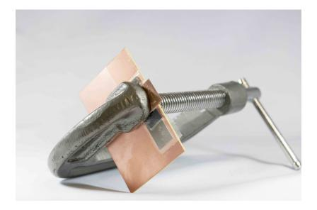
Figure 5-4: The clamped diode's construction.
