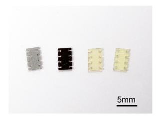
Figure 2-1: Insulating parts made from various materials: (left to right) fishpaper, polyester, polyimide, Garolite.
