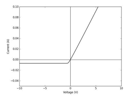
Figure 5-1: A simulation of a diode made with copper and aluminum.
