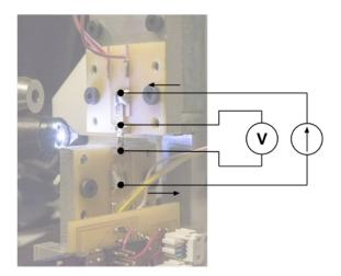
Figure 7-4: Joint cycling machine
