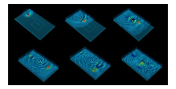
Figure 6-6: FDTD simulation of a spiral chip antenna.
