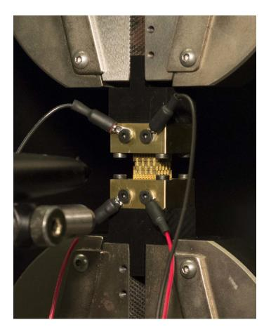
Figure 7-10: Bulk resistance test specimen in instron.
