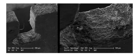
Figure 7-19: SEM micrograph of a slot that has been used.
