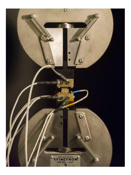
Figure 7-14: Temperature response fixture
