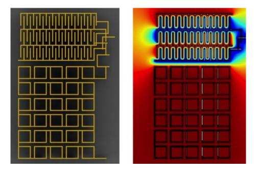
Figure 6-3: Electromagnetic modeling of LC resonator.
