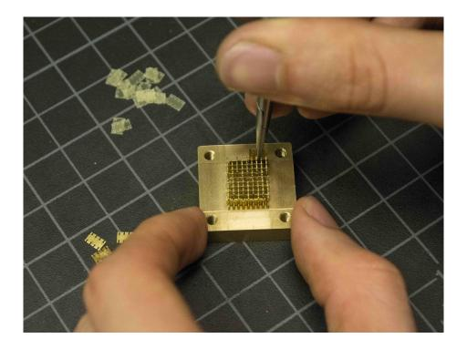
Figure 4-3: Assembling a discrete capacitor
