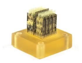
Figure 4-4: An epoxy substrate serves as an electrically insulating substrate.
