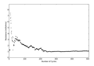
Figure 7-5: Resistance of joint vs number of cycles
