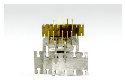
Figure 2-6: Hierarchy can be achieved through the use of adapter parts.
