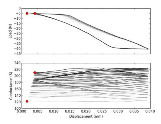
Figure 7-12: Plot of conductance/extension and load/extension loops over 20 cycles. The red circle denotes the start of the experiment and the red diagonal denotes the end.
