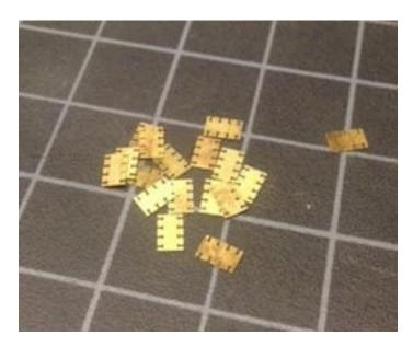
Figure 2-10: Brass parts milled on the Hurco
