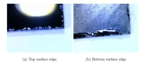
Figure 2-15: Showing close up of edge created by dicing saw. Some chipping is evident.
