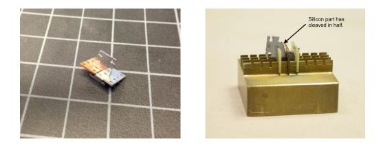
Figure 5-3: Two Schottky diode assemblies: a successful press-fit connection (left), a failed press-fit part insertion (right).
