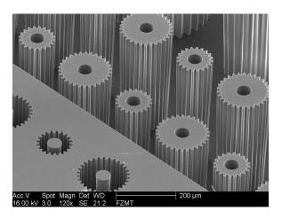
Figure 2-19: High aspect-ratio gears made with DRIE. [33]
