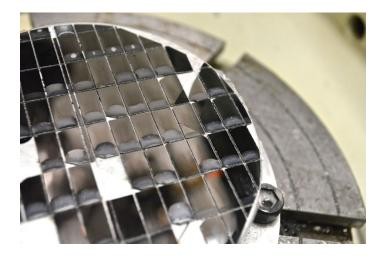
Figure 2-14: Close up of result of silicon wafer after dicing. Cracking is in the (001) > direction.
