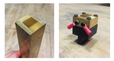
Figure 7-9: Bulk resistance fixture block.
