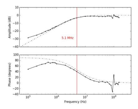
Figure 4-12: A bode plot showing amplitude and phase shift of a inductor.
