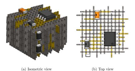
Figure 3-2: Discretely assembled circuit render.
