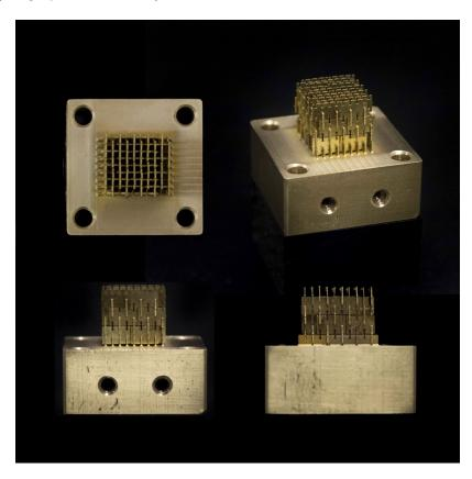
Figure 7-8: Bulk resistance test specimen.
