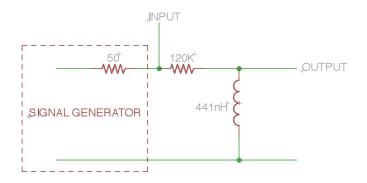
Figure 4-11: The RL circuit used to measure the frequency response of the inductor.
