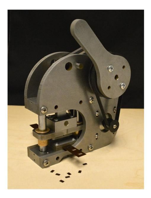
Figure 2-8: Custom punch press used to stamp parts
