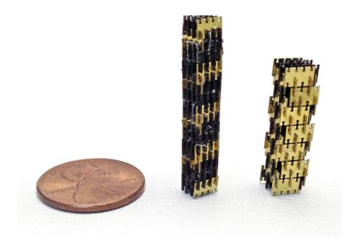
Figure 4-2: A discretely assembled inductor (middle) and capacitor (right) next to a penny for scale.
