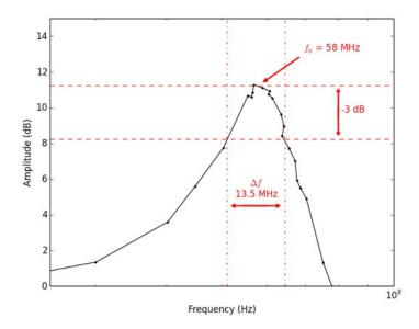
Figure 4-15: Q-Factor analysis of the LC Resonator.
