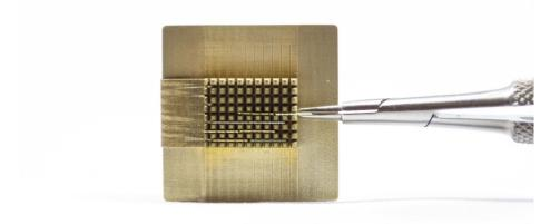
Figure 9-1: Parts are sequentially loaded into the rows of the pin array from the edge.
