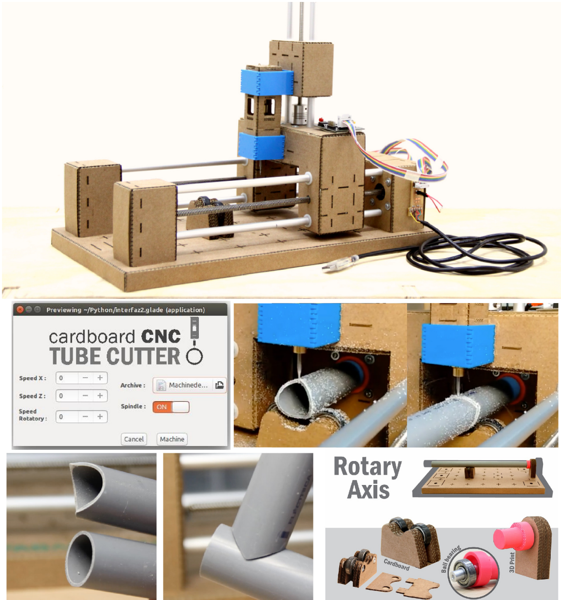
Figure 7-10: A cardboard CNC tube cutter designed by Fab Lab Tecsup students Fabio Ibarra, Gabriela Mojoli, Jesús Valencia, Roosvelth Cántaro, and Jorge Valcárcel. The machine uses a rotary axis to spin a tube, and a mill with two degrees of freedom to make precise cuts. Documentation available at http://archive.fabacademy.org/archives/2016/fablabtecsup/students/machinedesign/index.html , accessed June 2016.
