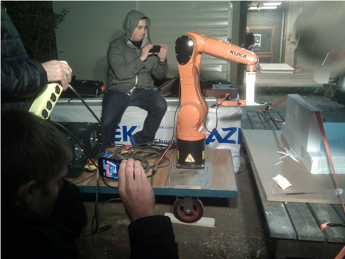
Figure 2-1: These are MIT architecture students using a 6-axis robot arm to cut complex surfaces into the foam block on the right. To create the toolpaths, they first designed the surfaces and Rhino, then used RhinoCAM to create instructions for the robot arm. The cutting end is an electric hot knife. To regulate the temperature of the hot knife, the student standing on the left is observing the cutting and flipping the switch on a surge protector on and off. This is an extremely intelligent controller for an extremely simple control task. However, despite these students being proficient at technologies such as CAD, CAM, and robot control, the system integration is tedious enough that the easiest way for them to get their system running was to incorporate an imprecise yet very expensive controller—a human.
