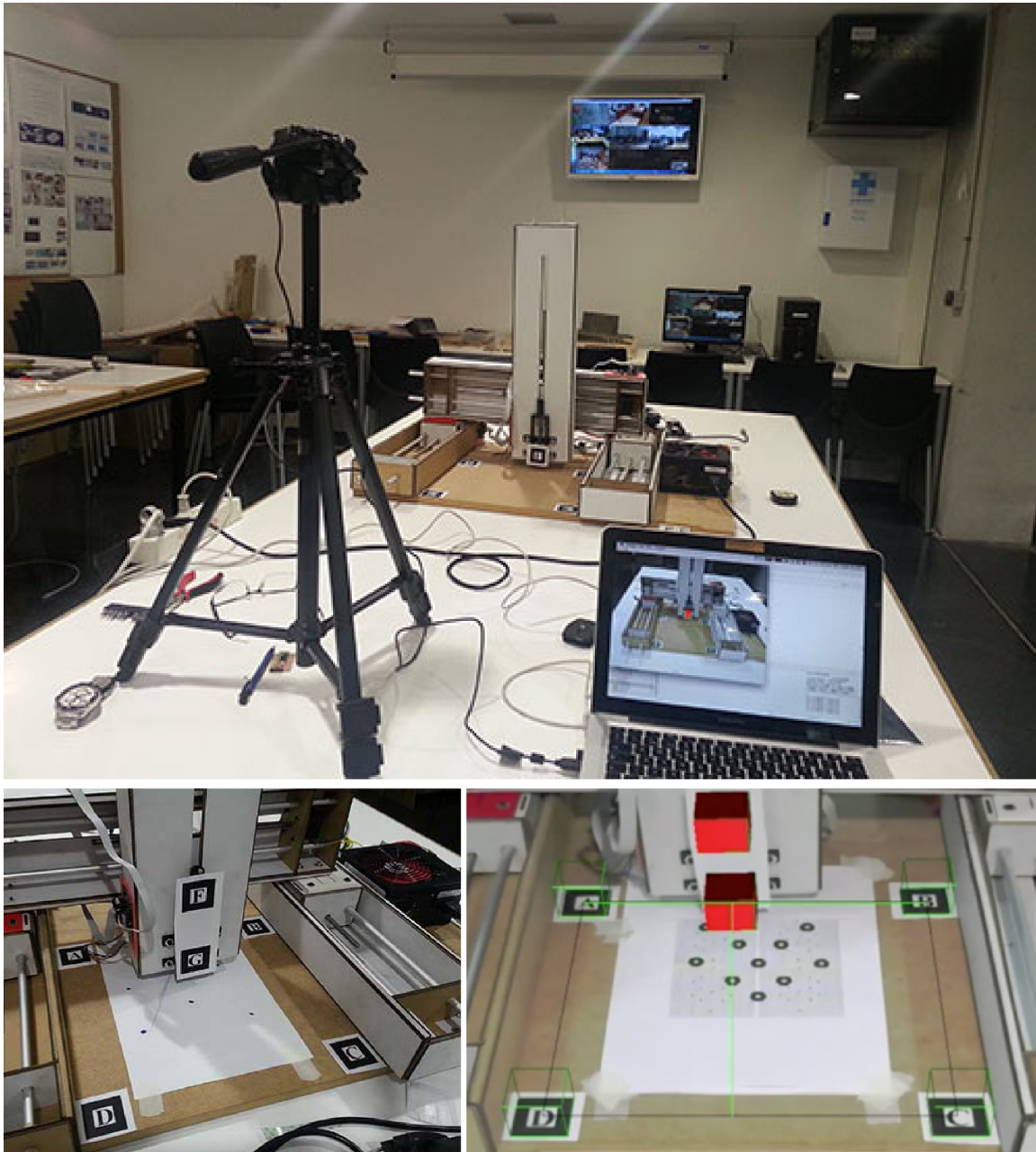
Figure 7-15: Cyclops: a machine that uses augmented reality markers for positioning. Cyclops was developed by Alejandro Escario-Mendez at Fablab Madrid. Additional documentation is available at http://fabacademy.org/archives/2015/eu/students/escario_mendez.alejandro/cyclops.html (accessed July 2016).
