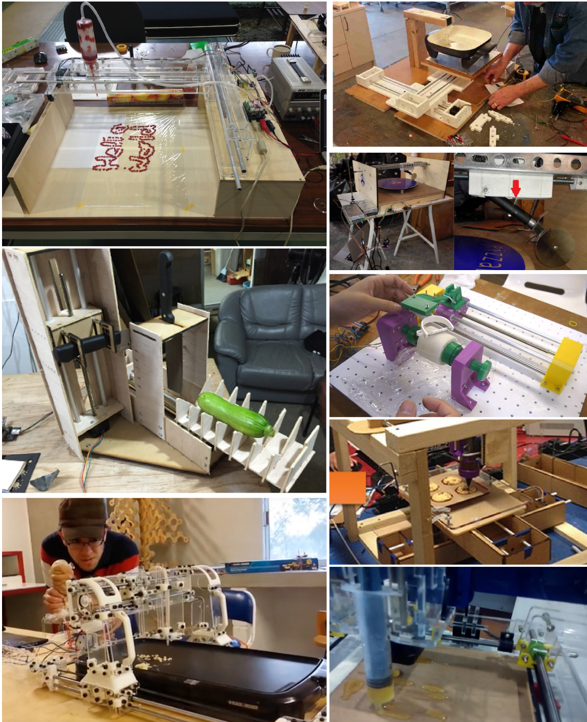
Figure 7-13: Many machines dealt with some aspect of food preparation. For example, clockwise from top left: a ketchup printer from Fablab Kitakagaya; a pancake printer from CITC Fablab Alaska; a pizza cutter from Fablab Barcelona; a vegetable peeler from Fablab Sendai; a cookie froster from AS220; a chocolate printer from Fablab Trivandrum; a vegetable cutter from Fablab Hamamatsu.
