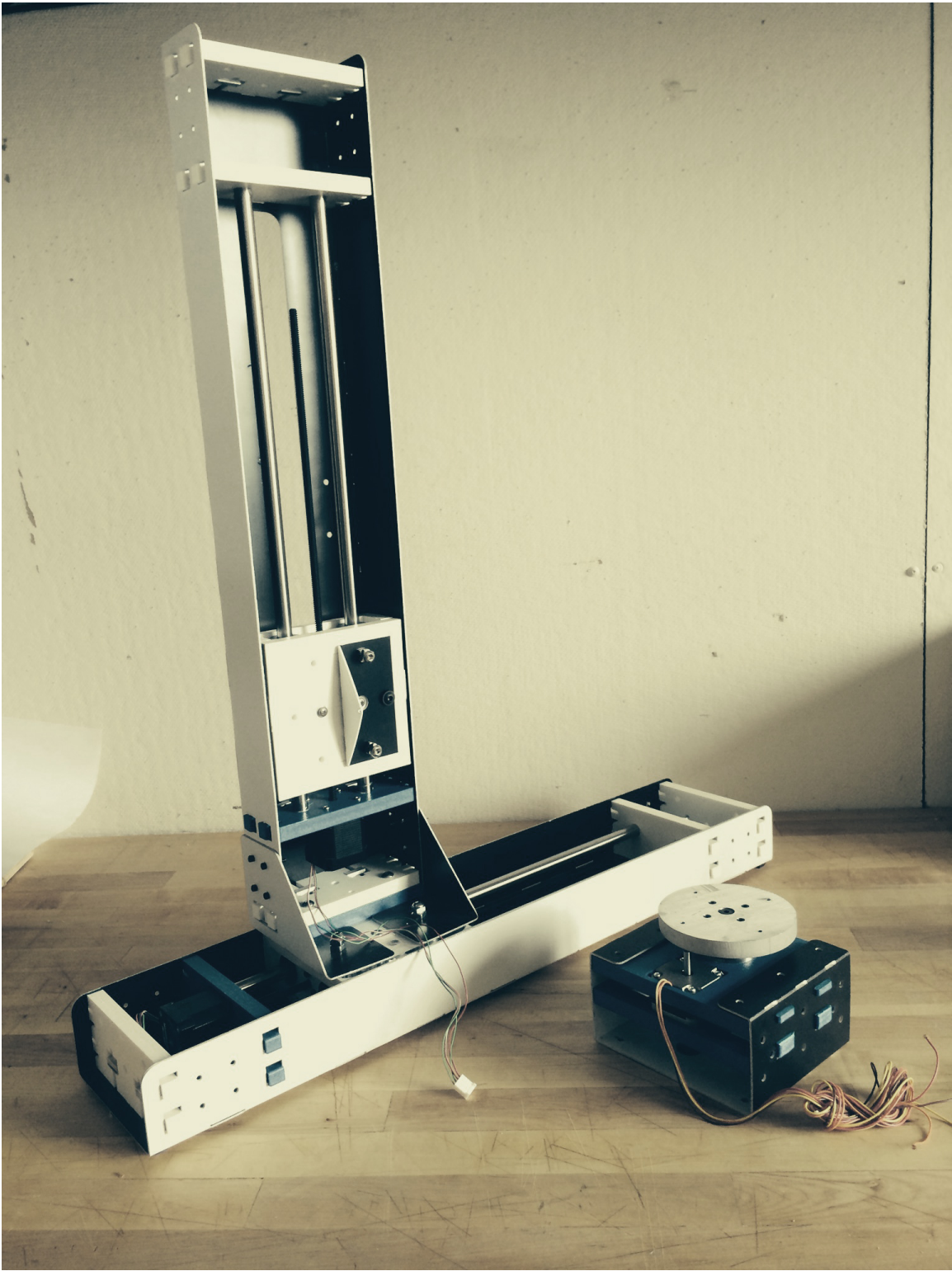
Figure 5-3: Two linear and one rotary stage, made of 1/16th aluminium and 1/2 inch HDPE.
