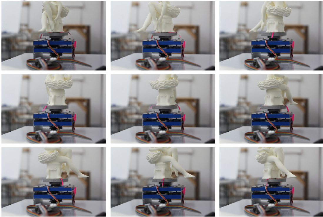
Figure 5-8: This is a machine that uses a rotary stage, a high-resolution camera, PyGestalt stepper nodes, and the mods workflow scripting environment to automate image capture. This imports a gphoto2 module as well as a PyGestalt VM into mods .
