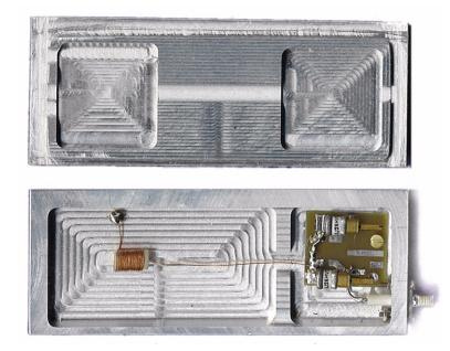
FIGURE 10.5.9 A single input single resonance probe for protons in an aluminum probe box designed and milled out using the IDEAS CAD program.
