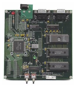
FIGURE 10.5.12 Hitachi evaluation board used for pulse programming and system control.
