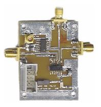
FIGURE 10.5.10 Photograph of the actual timing distribution circuit that takes a 40 MHz reference from the HP E1445A, divides it down to 20 MHz and 10 MHz references to be used by other parts of the system. The full schematic can be found in appendix E.
