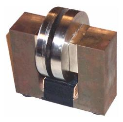
FIGURE 10.3.4 A 13 lb. permanent magnet used for the spin echo experiment. Homogeneity is 100-1000 ppm.
