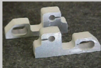
An example of two aluminum parts done in 1/2" (1.3 cm) thick aluminum, which took approximately five minutes machine
