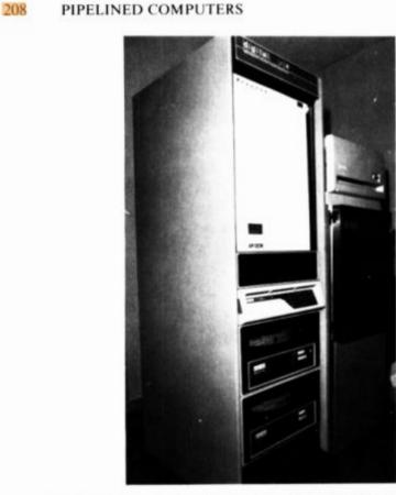
FIGURE 2.36 An overall view of an FPS AP-120B installation. The AP-120B occupies only 29 inches of rack space, and is attached to a PDP 11/34 with two disc units, a tape reader and output printer. The control teletype or VDU is not shown. (Photograph courtesy of D Head and Floating Point Systems, S A Ltd.)
