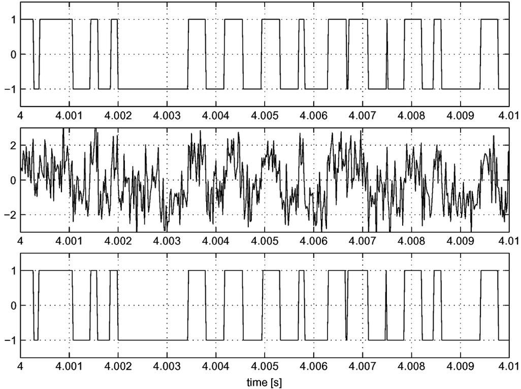
Fig. 10. Top: example of pseudorandom signal  $\hat{X}(t)$  generated by the circuit of Fig. 9. Middle: noisy signal  $Y(t)$  as in Fig. 9 at SNR = 0 dB. Bottom: measured output signal  $\hat{\hat{X}}(t)$  of the circuit of Fig. 11 fed with  $Y(t)$ .
