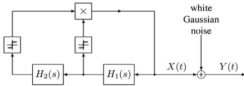
Fig. 9. Continuous-time analog to Fig. 1 with low-pass filters instead of delay cells.
