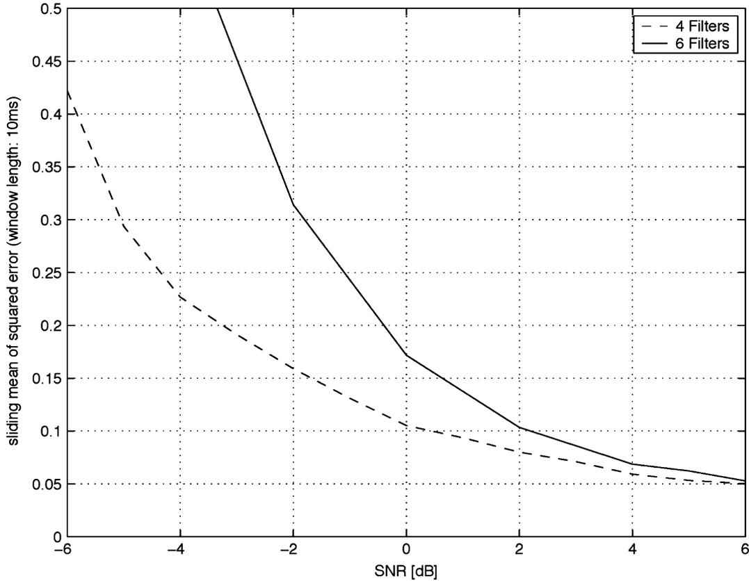
Fig. 14. Average squared error in steady state versus SNR. Dashed curve: pseudorandom signal with shorter period (7 ms instead of 34 ms, achieved with  $H_2(s) = H_1(s)^4$  instead of  $H_2(s) = H_1(s)^6$ ).
