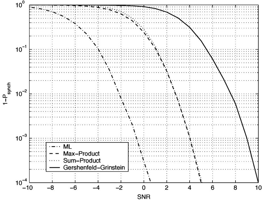
Fig. 8.  $1 - P_{\text{sync}}(k = 100)$  versus SNR for the LFSR with  $m = 15$  ( $\ell = 1$ ). Algorithms (in the order of increasing performance): G.-G. soft LFSR [3]; sum-product soft LFSR; max-product soft LFSR; maximum likelihood (ML).
