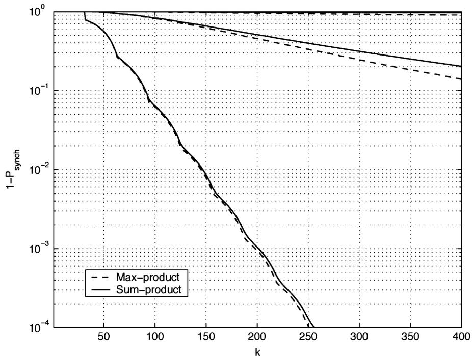
Fig. 7.  $1 - P_{\text{sync}}(k)$  for the LFSR with  $m = 31$  ( $\ell = 3$ ) for three different signal-to-noise ratios:  $\text{SNRs} = -2.92$  dB ( $\sigma = 1.4$ ),  $\text{SNR} = 0$  dB ( $\sigma = 0$ ), and  $\text{SNR} = 4.44$  dB ( $\sigma = 0.6$ ). Algorithms: max-product soft LFSR and sum-product soft LFSR.
