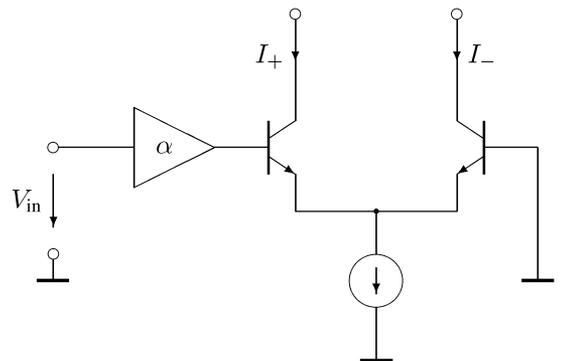
Fig. 12. Differential transistor pair used for blocks ①, ②, and ⑤.
