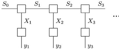
Fig. 2. Factor graph (Forney-style) corresponding to the trellis of the system in Fig. 1.
