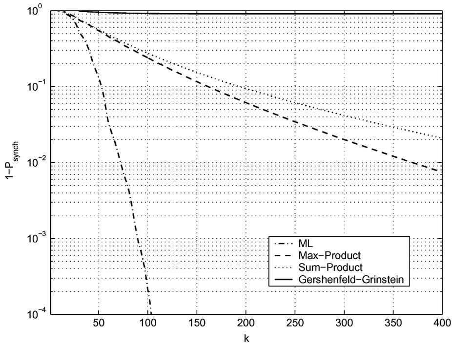
Fig. 6.  $1 - P_{\text{sync}}(k)$  for the LFSR with  $m = 15$  ( $\ell = 1$ ) at  $\text{SNR} = 0$  dB. Algorithms (in the order of increasing performance): G.-G. soft LFSR [3]; sum-product soft LFSR; max-product soft LFSR; maximum likelihood (ML).
