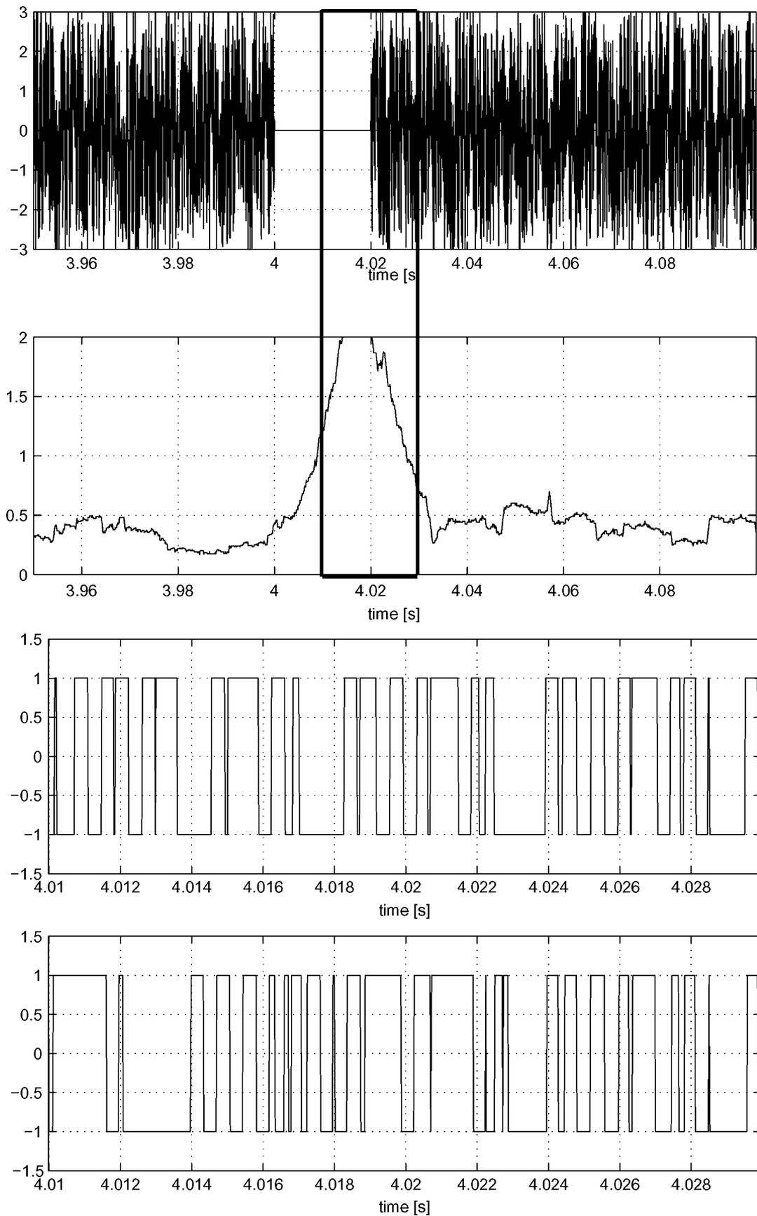
Fig. 15. Resynchronization example with modified  $Y(t)$  (top), sliding-window squared error (2nd from top),  $X(t)$  (2nd from bottom), and  $\hat{X}(t)$  (bottom) at SNR = 0 dB. The plots of  $X(t)$  and  $\hat{X}(t)$  are zoomed to the marked interval around  $t = 4.02$  s.
