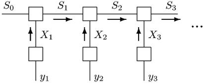
Fig. 3. Forward-only message passing through the factor graph of Fig. 2.
