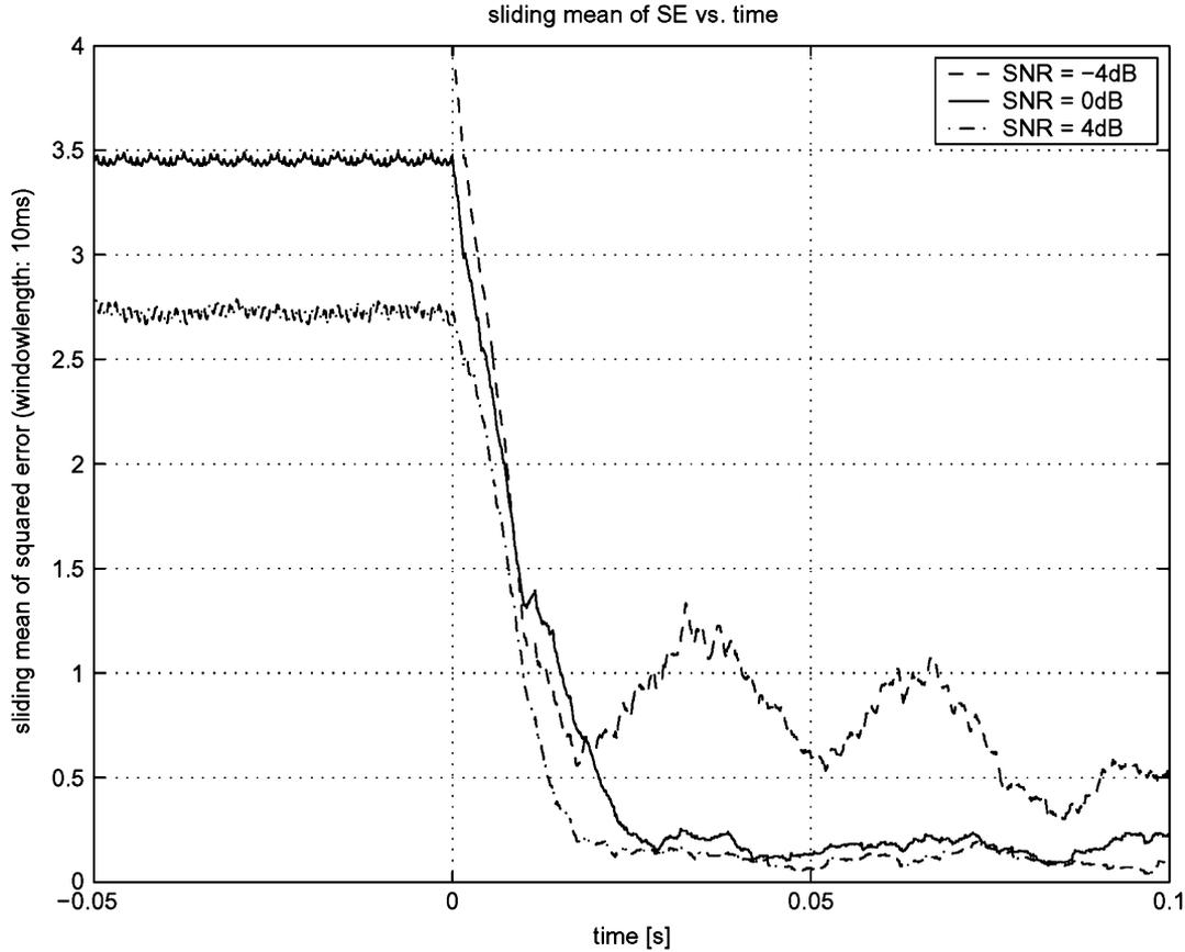
Fig. 13. Average squared error versus time after switching the transmission on.
