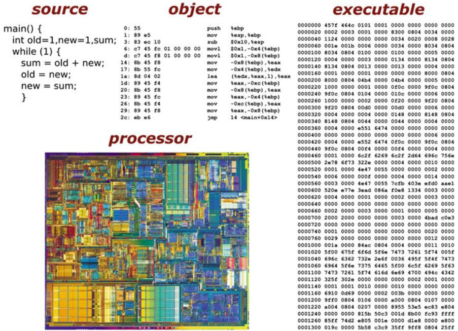
Fig. 1 Conventional representations of the calculation of Fibonacci numbers
