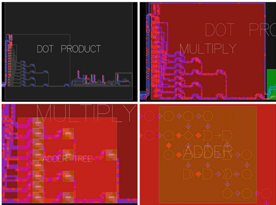
Fig. 5 Hierarchical structure of a zoom through an ALA dot product [24]
