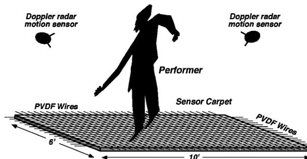
Figure 1: Sensor Arrangement for the Carpet System
