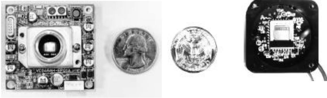
Figure 4: Two of the small, inexpensive, monochrome video cameras tested for VSM application; the CX-103 (left) and VVL Peach (right).
