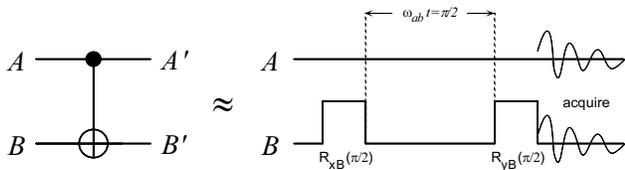
FIG. 5. Quantum circuit symbol for a controlled-NOT gate, and its implementation with RF pulses in our two-spin NMR system in the doubly degenerate frame. The time  $\pi/2\omega_{AB}$  was 2.326 milliseconds in the experiment.
