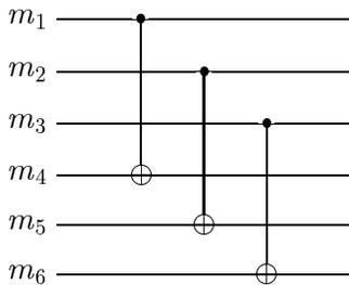
FIG. 2. Network of CNOT’s to move zeros for 3 pure qubits  $m_{1,2,3}$  conditioned on 3 ancilla  $m_{4,5,6}$ .
