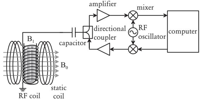
FIG. 4. (B) Schematic of an NMR apparatus.
