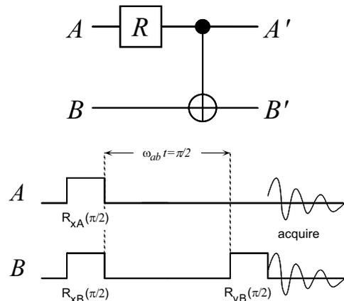
FIG. 6. (top) Quantum circuit, where the boxed  $R$  denotes the single-qubit rotation  $\hat{R}_x(\pi/2)$ , and (bottom) corresponding pulse program for creating an EPR state.
