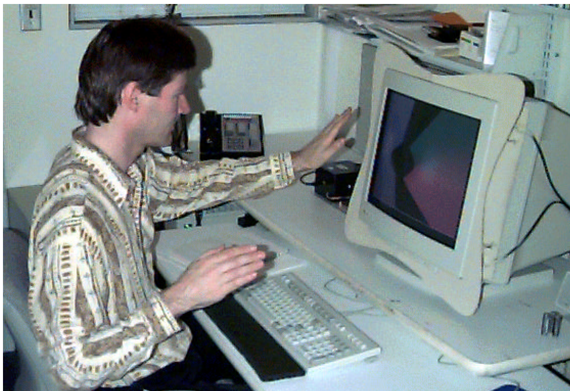
Figure 2: The “Flying Fish”; navigating through a virtual world by moving hands around a monitor screen. The user sits on a transmitting electrode atop his chair; the receive electrodes can be seen at the edges of the monitor
