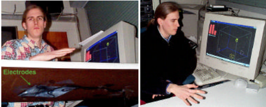
Figure 5: A “Smart Table”. Electrodes below (seen under the table in the left figure) sense the position of a hand above, allowing free interaction with a simple virtual environment, visible on the monitor
