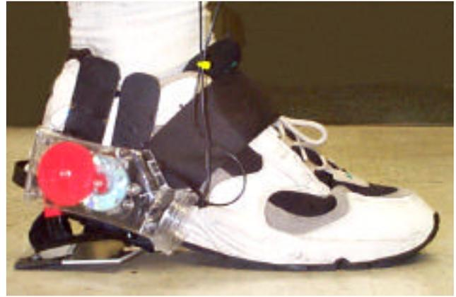
Figure 6: Simple shoe-mounted rotary magnetic generator
