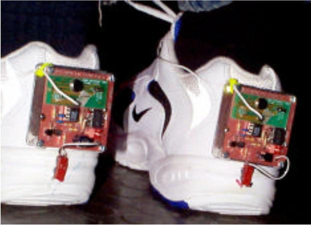
Figure 14: A pair of self-powered RFID sneakers
