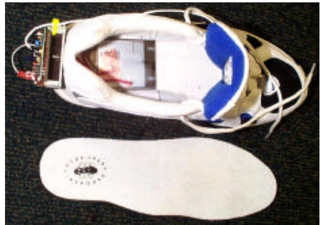
Figure 11: Sneaker-mounted tag circuitry and PZT element
