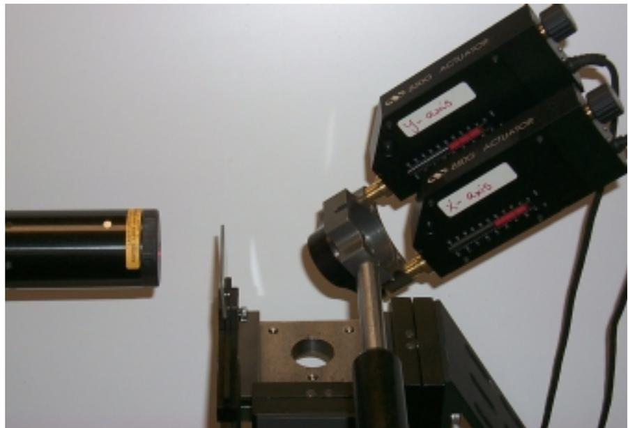
FIGURE 7.9 TWO VIEWS OF THE LASER POSITIONING SYSTEM
