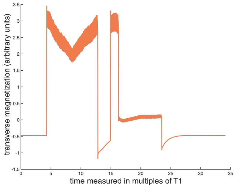
Figure 6-5: Spelling out the letters “ML” in the envelope of the spins. This takes place over many  $T_1$  and shows how controllability is successful when the maximum  $X$  target is kept less than or equal to  $1/2$
