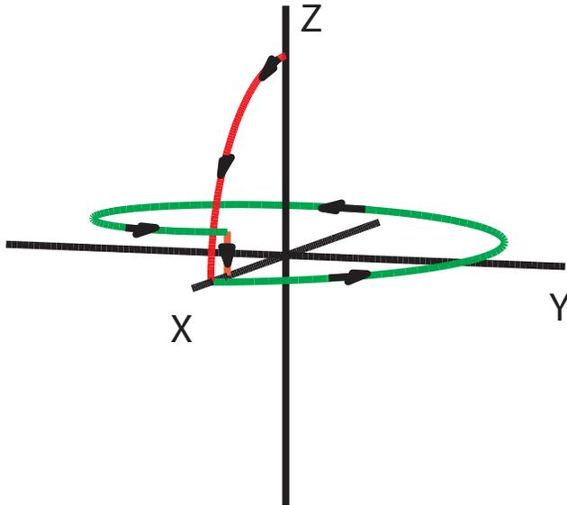
Figure 5-1: The idea behind unitary correction. Suppose we want to keep the Bloch vector in the x-y-plane. We first rotate the vector into the x-y-plane (the red path). The vector spins about the z-axis and relaxes (the green path). Then we try to push it back into the x-y-plane (the orange path). Such a procedure will result in a steady state Bloch vector.
