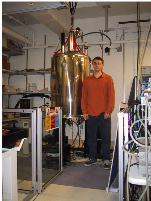
Figure 5-20: 500MHz superconductor magnet with Jason for scale
