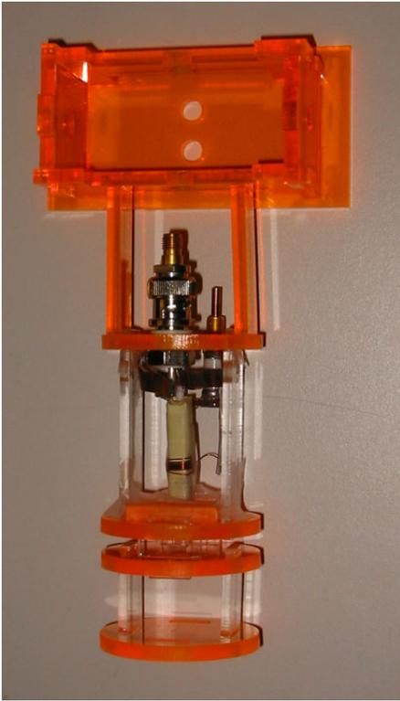
Figure 5-11: Halbach cylinder probe; created by Isaac Chuang
