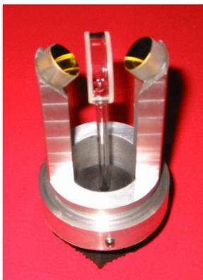
Figure 5-13: Sample holder with mirrors; Design and construction by Daniel Benhammou, MIT
