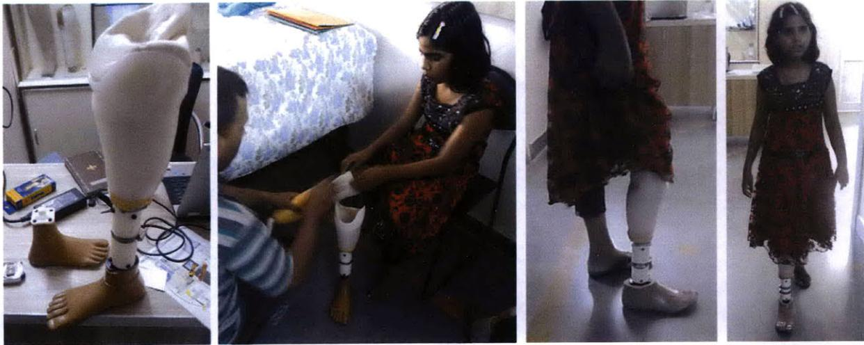
**Figure 7.34:** Patient testing the extension prostheses. The Jaipur foot is only available with a relatively high ankle block (see feet on left), leaving little room for the pylon and its extension. Finally we tested the extension pylon with a low-profile SACH foot (right).
