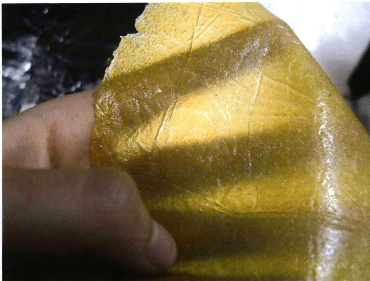
**Figure 7.3:** *The soy protein polymer sheet was pressed between two sheets of aluminium foil in a hot press. The aluminium foil was slightly wrinkled, which caused the lines and texture.*
