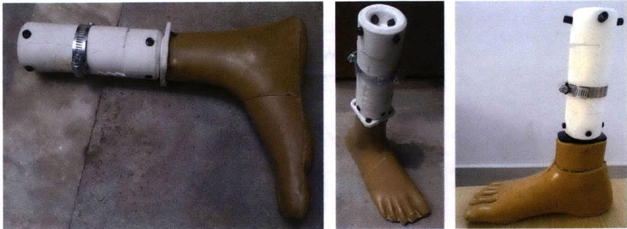
**Figure 7.32:** Extension pylon attached to two different paediatric Jaipur feet. The first has a very high ankle block, and the pyramid that is attached to it is too large for ankle. The second has a locally manufactured cast metal pyramid, but that pyramid is only screwed in in the centre, causing rotational play.
