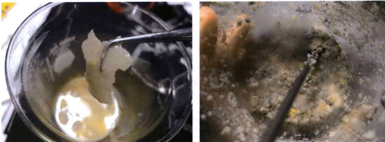
**Figure 7.4:** *Submerging the protein film into water would cause it to disintegrate within a matter of hours. Uncured protein granules left at my desk for more than 2 days would start moulding abundantly.*
