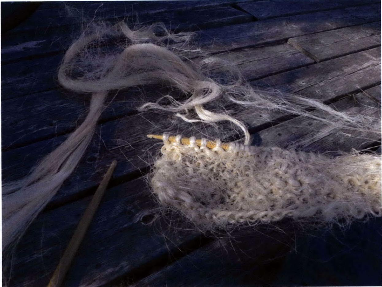
**Figure 7.16:** Because of the lack of woven or knit structural natural fibres (like sisal, which in strength is comparable to fibreglass), this was an exercise in getting long sisal fibres into a sheet. The hand-knitted sisal unfortunately did not have uniform stretching properties. However, if knit with more care, knit natural fibres could be useful in making sheets that can attain non-zero Gaussian curvature during composite lay-up.
