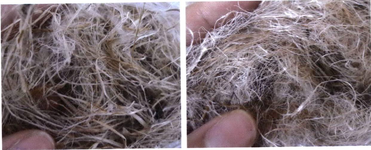
**Figure 3.4:** Left: Raw hemp fibres from Hemp Traders Ltd. in Santa Monica, CA, Right: Washed kenaf fibres, FK100 DSAT 50mm fibres from Bast Fibres LLC New Jersey.
