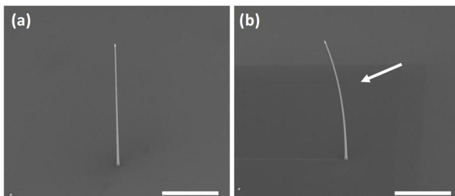
Figure 3.17 Low dose ion implantation (a) before and (b) after irradiation. Beam incidence from right side as indicated by arrow in (b). Scale bars: 5 μm.
