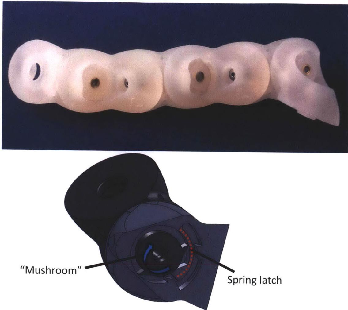
Figure 4.6: Photograph and CAD rendering of cut-away view of single-position latching stochastic Motein.
