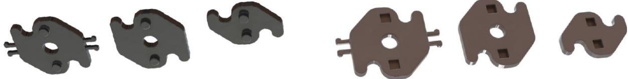
*Figure 55 Parts after molding re-design. (L) Positive side with protruding pegs (R) Negative side showing cavity.*
