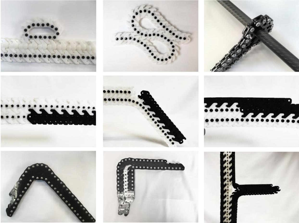
Figure 28 Structural primitives. On the top row strands are shown locking to themselves. The middle row shows a break in a strand and connector strands. The bottom row shows controlled angles.
