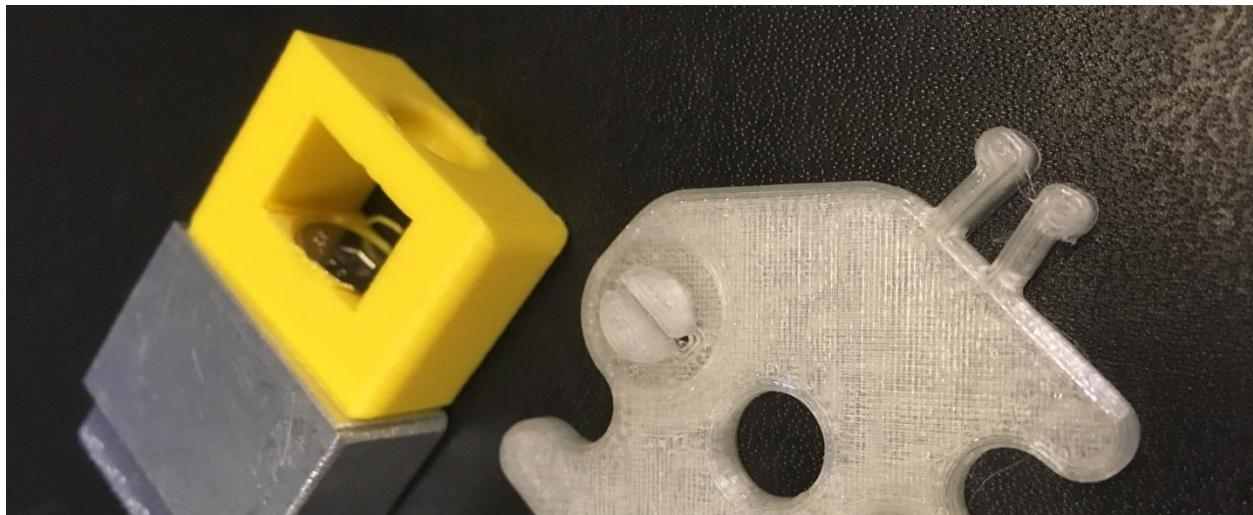
Figure 78 PLA failure during side snap tensile test. Notice the peg is permanently bent inward.
