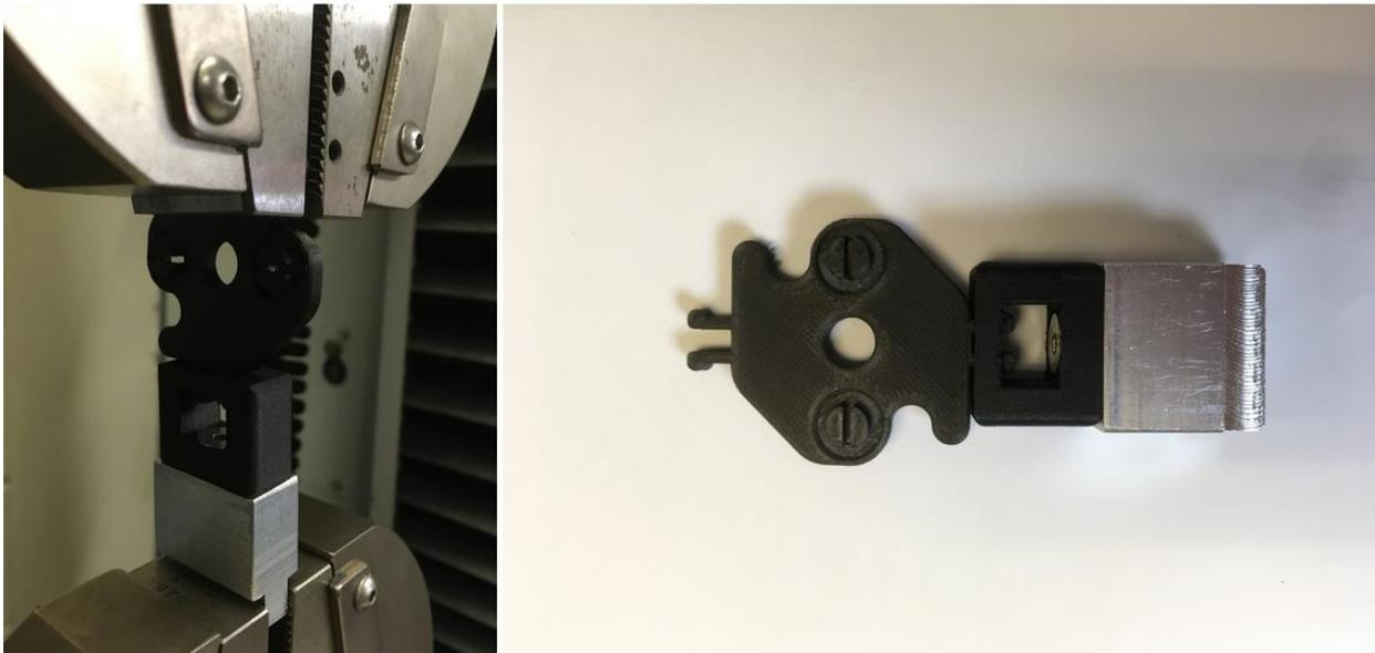
Figure 77 Experimental set up for side snap tensile tests.
