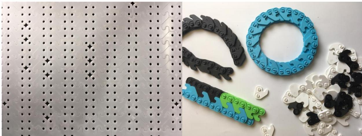
Figure 49 2D laser cut sheets and 3D printed parts
