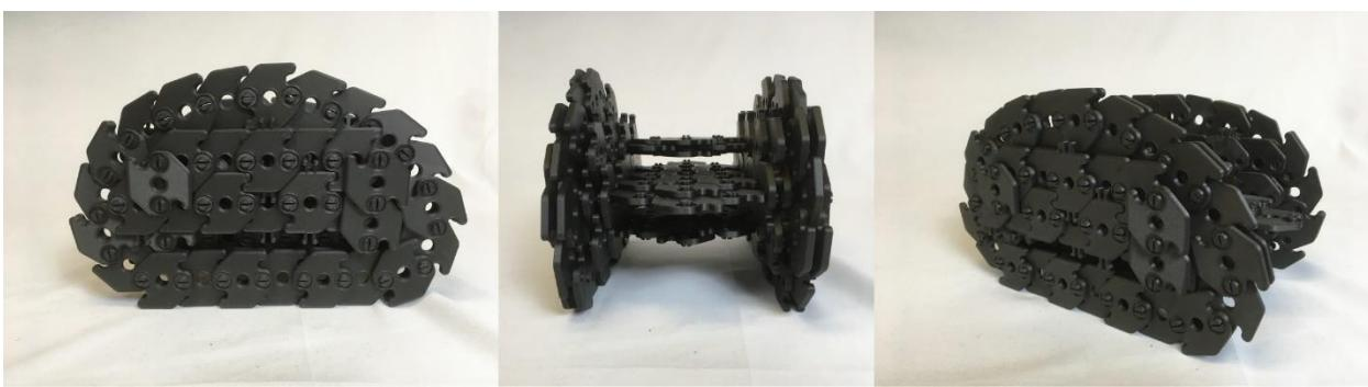
*Figure 68 Prototype toy vehicle whose tracks can rotate freely.*
