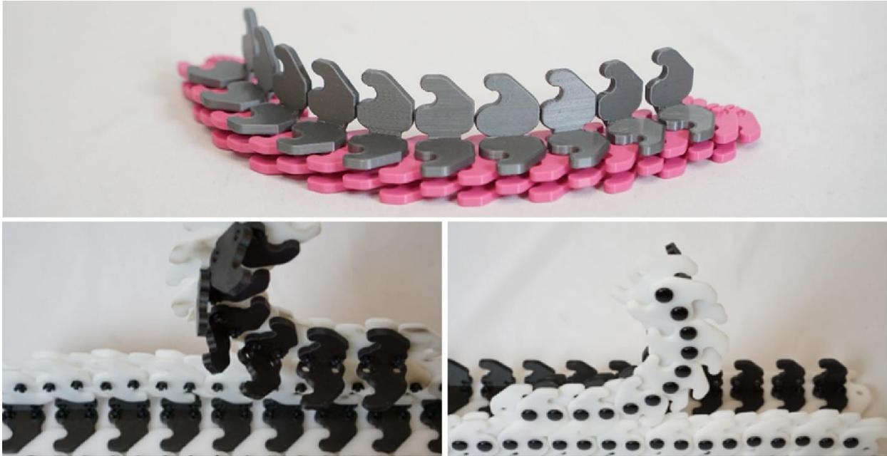
Figure 37 (Top) Angled strand fabricated with snaps (Bottom) Angled strands fabricated for the rivet-based system shown zipping to a structure
