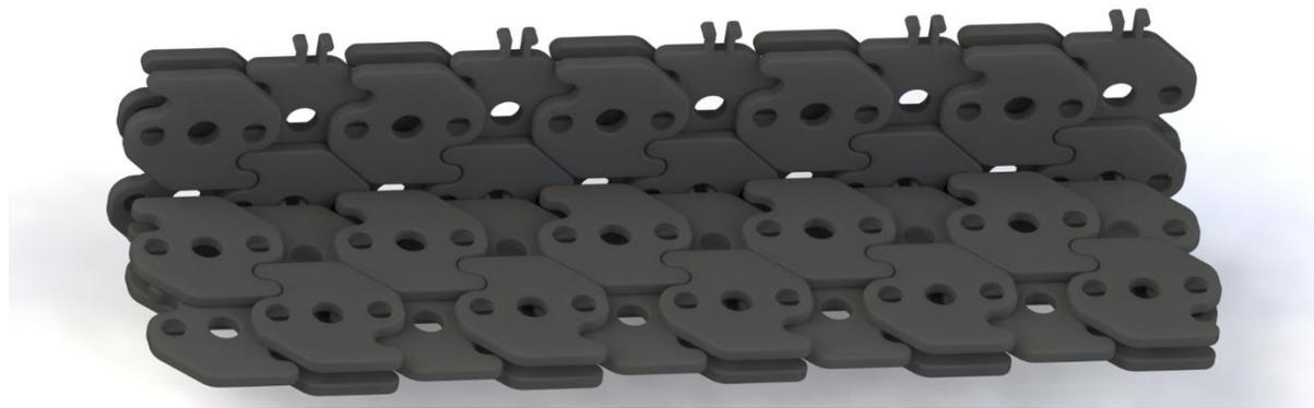
Figure 31 Side snaps connecting two sheets
