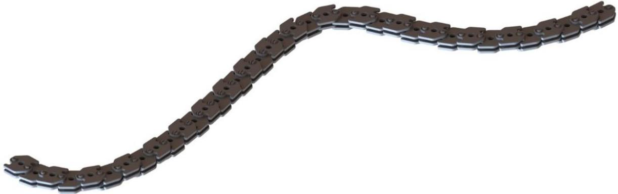
Figure 24 Chain of zipped elements, not constrained and thus flexible in plane.
