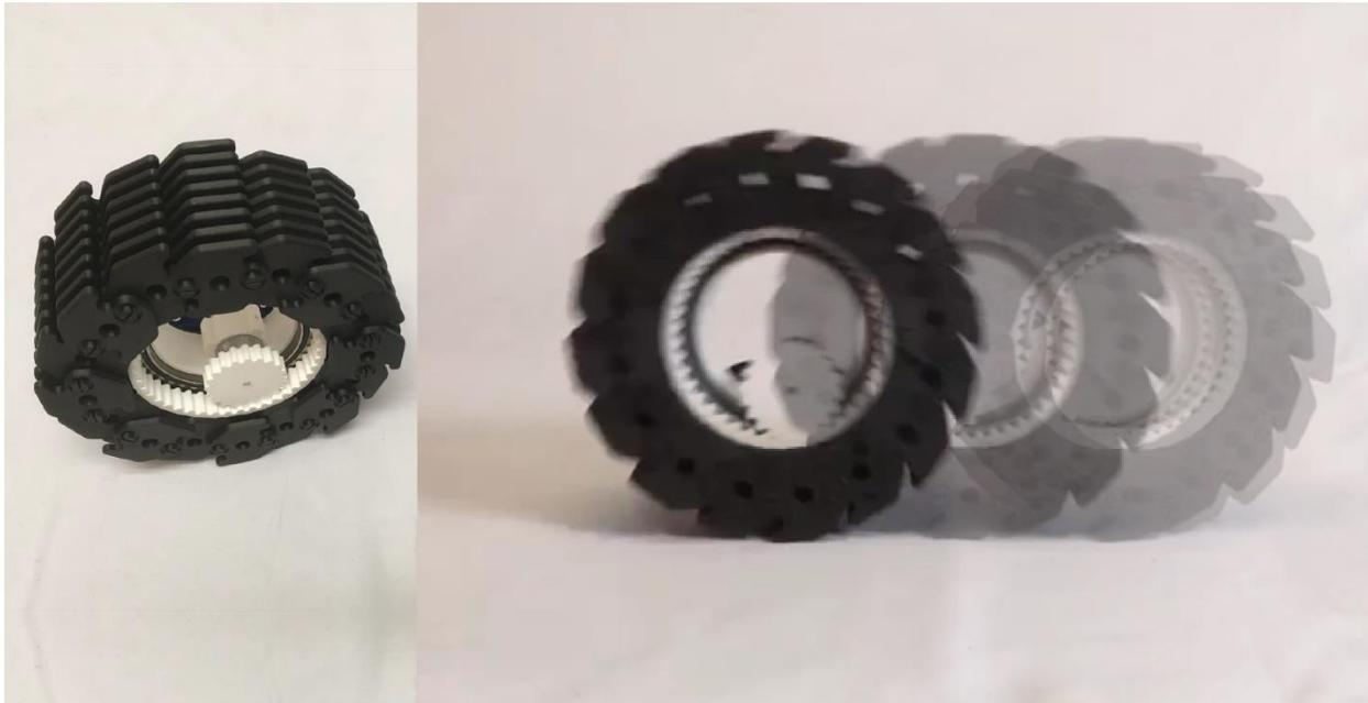
*Figure 67 Hamster wheel robot constructed from Zipped pieces which can self-locomote*
