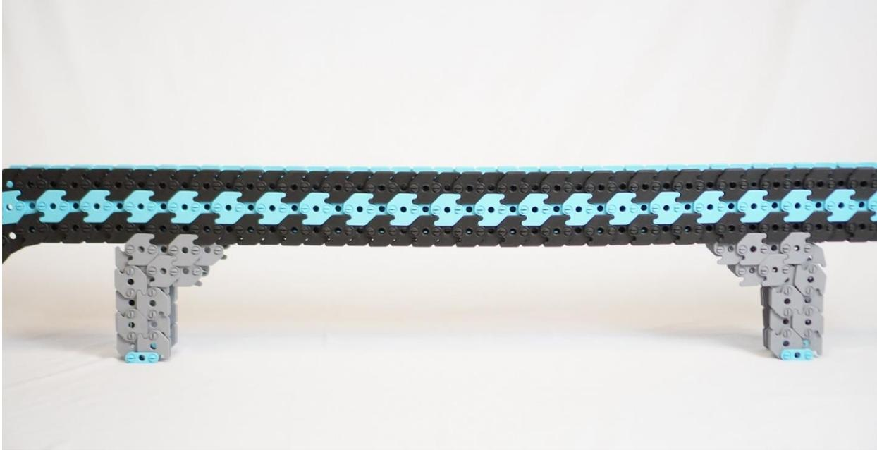
Figure 71 Hand-built beam bridge spanning a 1m gap.
