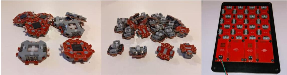
Figure 2-2: Meso-DICE components. Left: nodes; Middle: struts; Right: build plate
