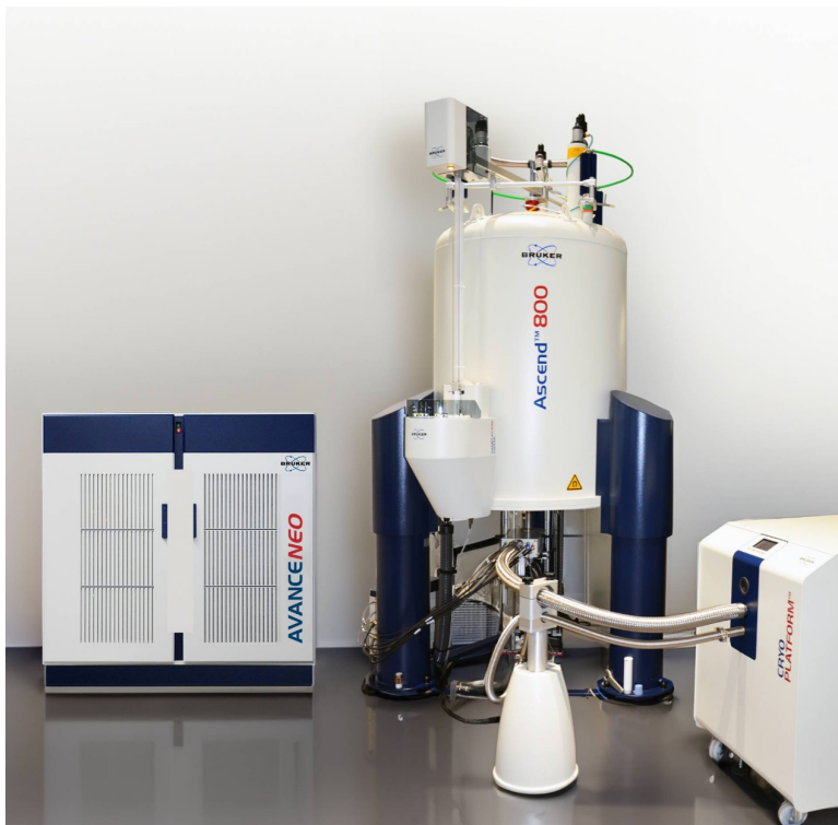
Figure 2.1: Bruker BioSpin AVANCE NEO console and Bruker Ascend 800 MHz NMR magnet at Francis Bitter Magnet Lab, used as the high-field experimental context for the diamond MAS-NMR rotor work.
