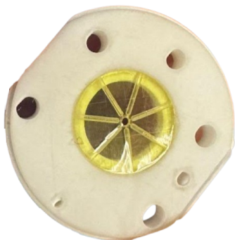
Figure 2.27: BMF-printed air-bearing and stator prototype components used to evaluate sub-millimeter bearing geometry and feed-channel resolution.
