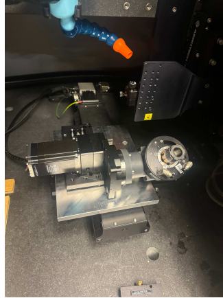
Figure 2.18: Through-bore air-bearing flip-spindle micro-lathe used for registered two-sided rotor machining.
