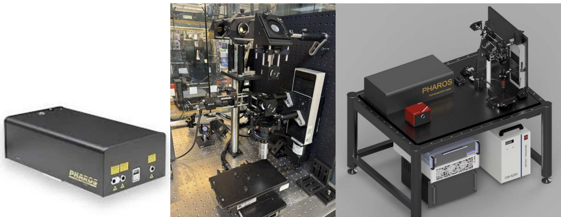
Figure 4.2: In-house femtosecond micromachining platform, showing the ultrafast source, optical table, beam-delivery optics, vertical optical breadboard, objective/imaging path, motion stage, chiller, and supporting electronics.
