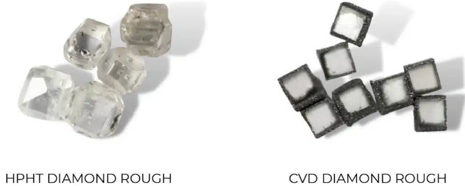
Figure 2.4: Typical rough single-crystal diamond morphologies from HPHT and CVD growth. HPHT rough is commonly faceted; CVD rough is commonly square or plate-like because it grows on a planar seed.
