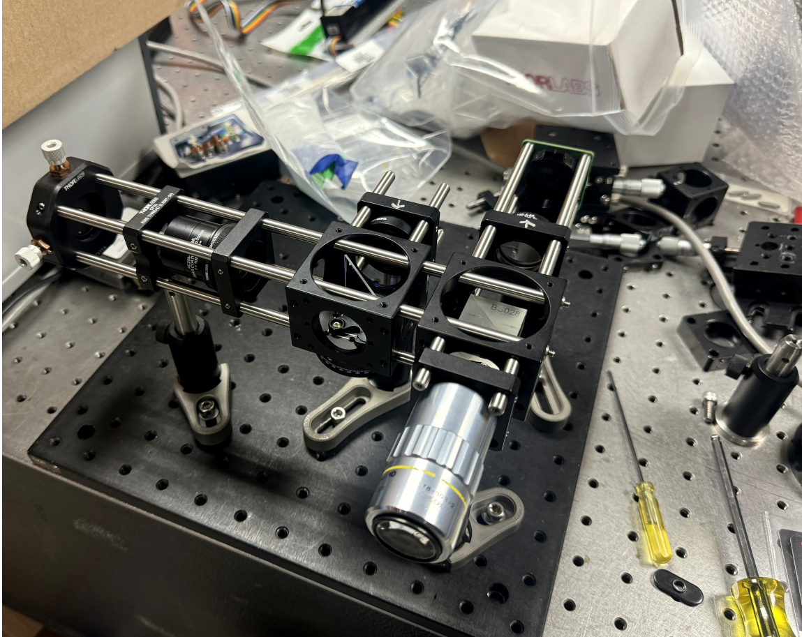
Figure 5.4: Bench implementation of the local Raman optical path during development. The system uses cage-mounted optics so the excitation, imaging, filtering, and spectrometer-coupling paths can be modified and realigned during iteration.
