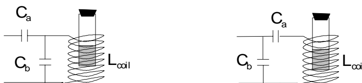
Figure 7.2: Two possible configurations for a probe circuit. The one on the left uses a capacitor in series with a capacitor in parallel with the coil. The one on the right uses a capacitor in parallel with a capacitor connected in series with the coil. The two configurations are equivalent.
