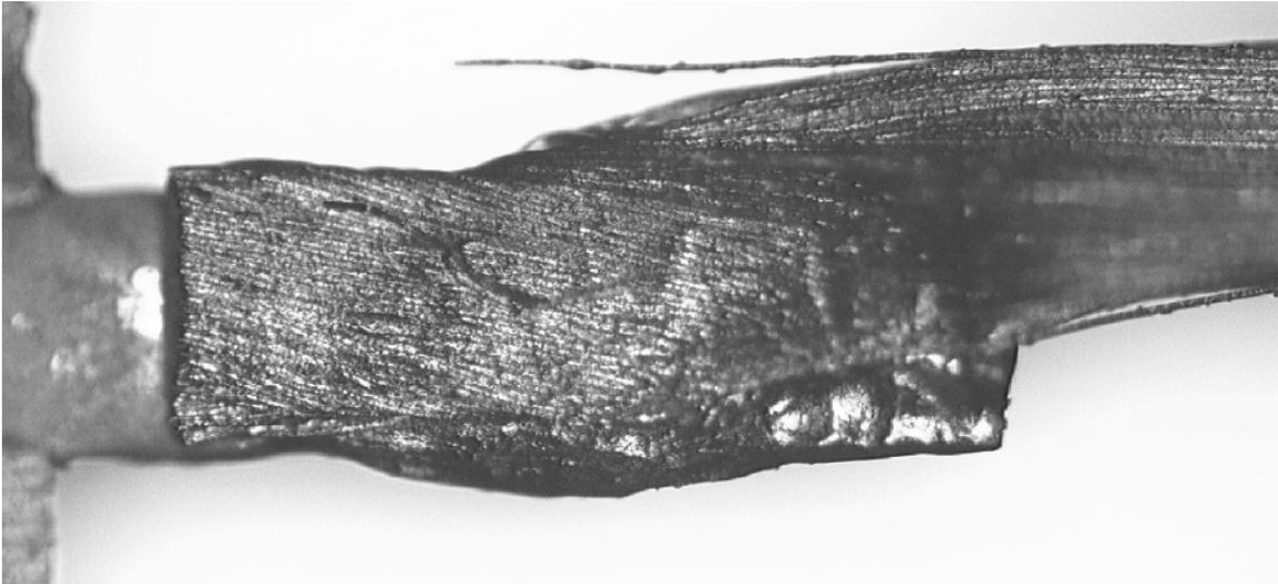
Figure 3.11: Top view of a stainless steel thread welded to  $Cu/CuSnPb$  lead.
