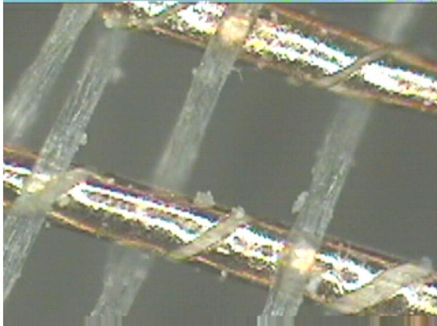
Figure 3.3: Micrograph of metallic organza.
