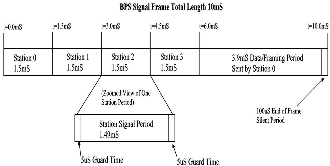
**Figure 6-1: BPS Signal Frame Timing**
