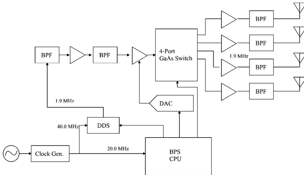
**Figure 9-1: BPS Transmitter Block Diagram**
