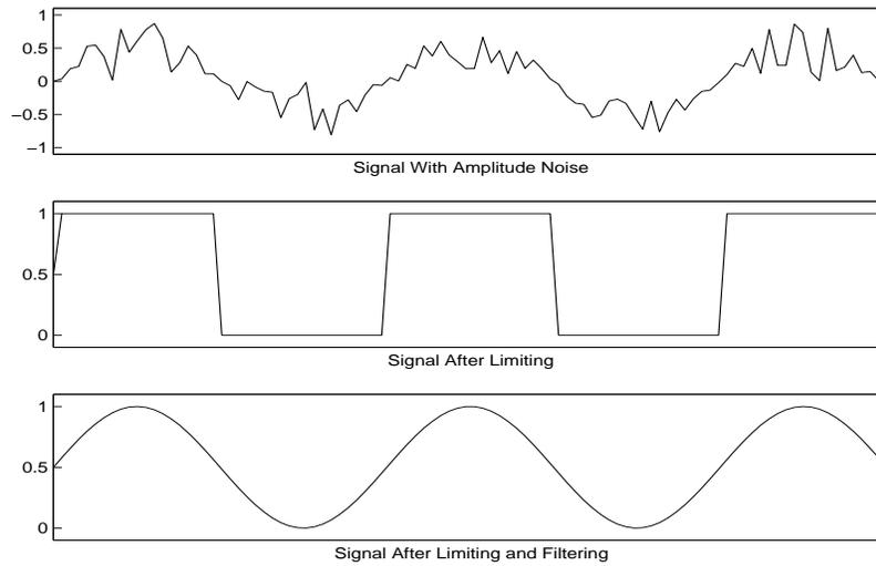
**Figure 8-2: Signal with AWGN During Processing**
