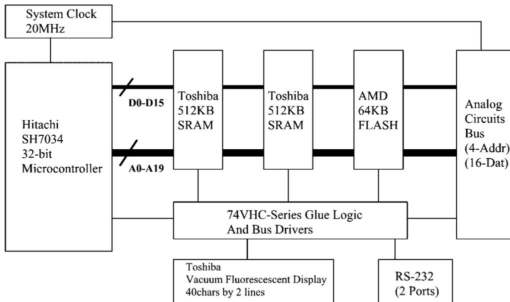
**Figure 8-3: The BPS CPU Module**
