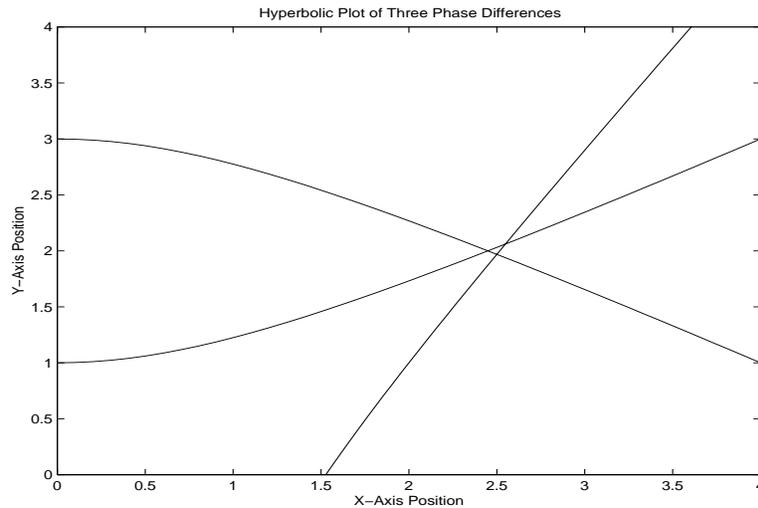
**Figure 5-5: Position Solution by Intersecting Hyperboloids**
