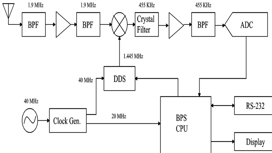
**Figure 8-1: BPS Receiver Block Diagram**
