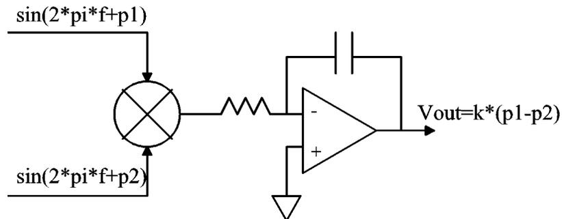
**Figure 5-3: Analog phase detector circuit**
