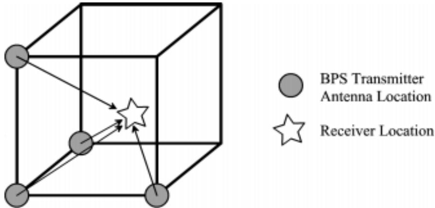
**Figure 5-1: Placement of Transmitters and Receiver**
