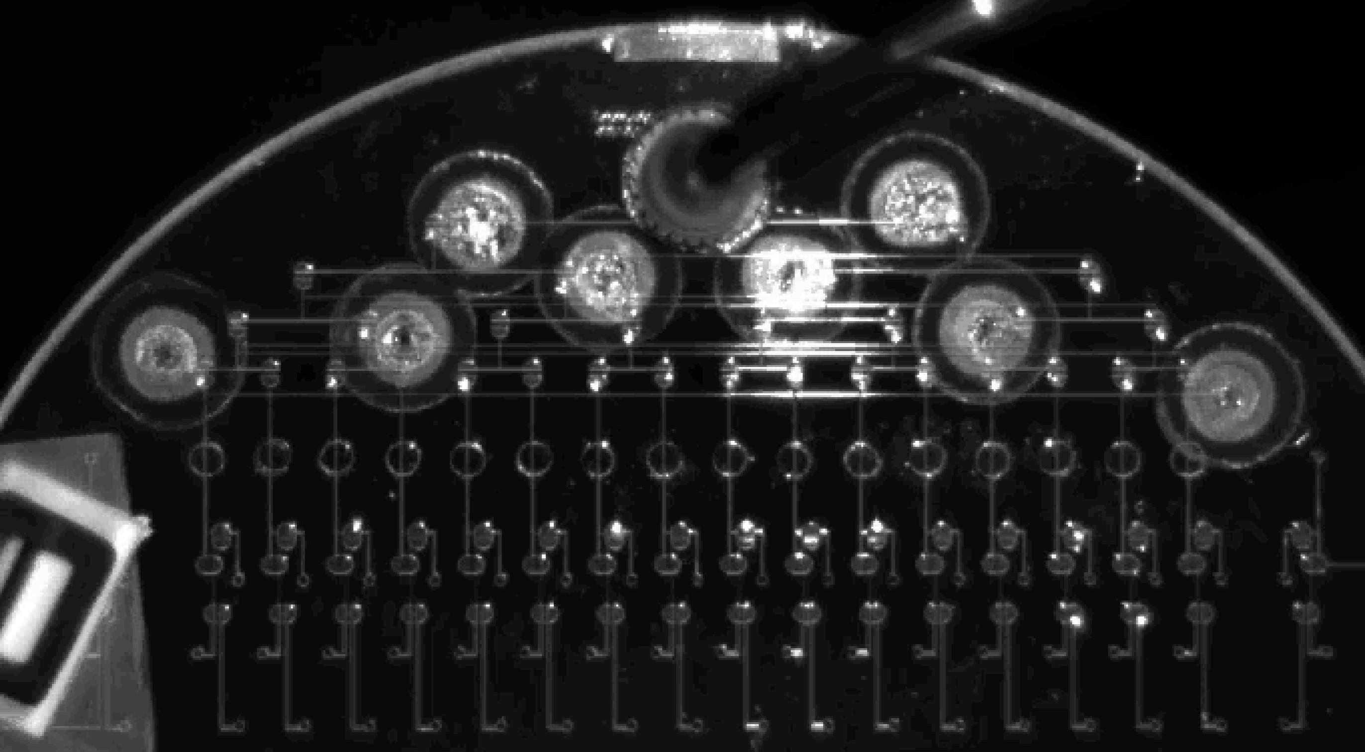
Set all 16 latching valves according to any pattern every **2 seconds**
