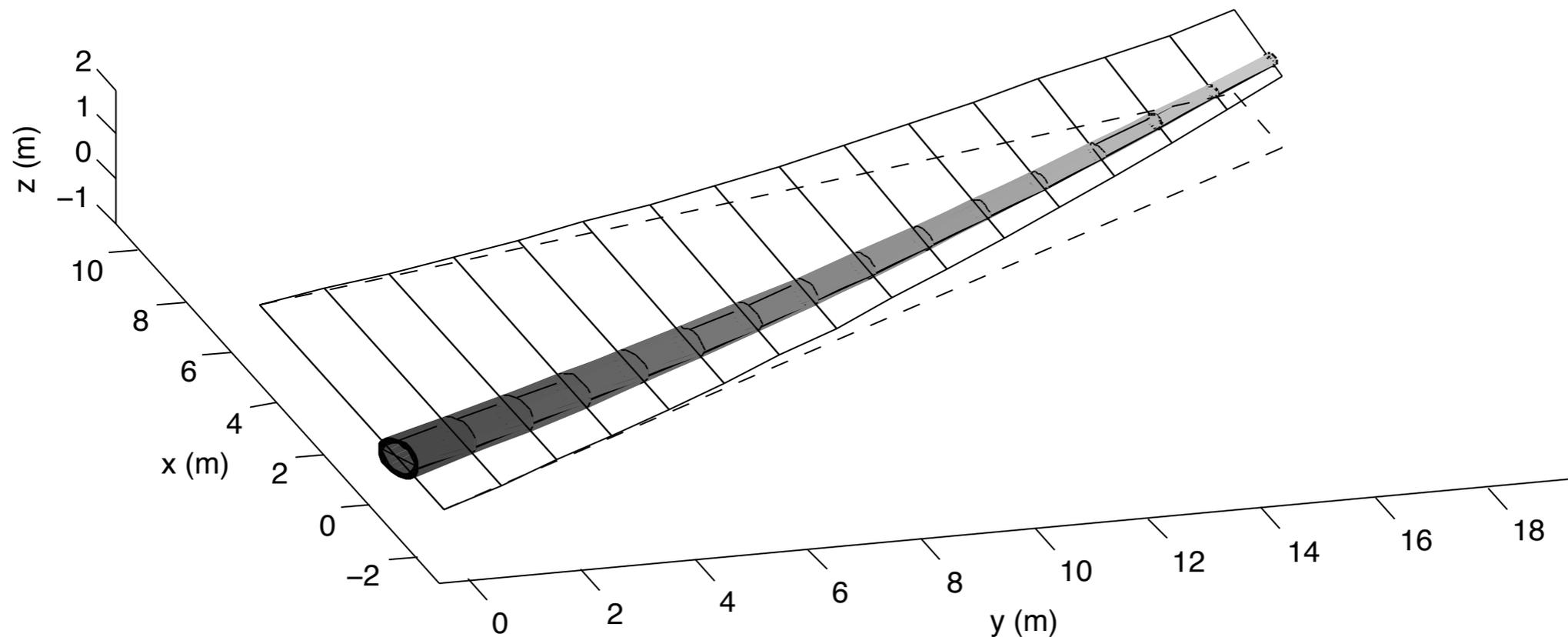
**Aerodynamics:** Panel code computes induced drag. Variables: **wing twist** and **angle of attack**
