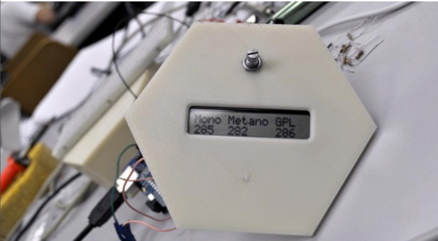
**A safety modular system featuring a beehive shape for embedding customised behaviours and sensors connected to internet**
