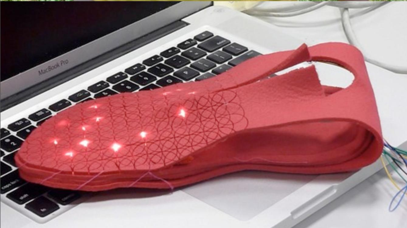
**A smart slipper made by laser cut acrylic felt providing feedback if the user steps incorrectly**
