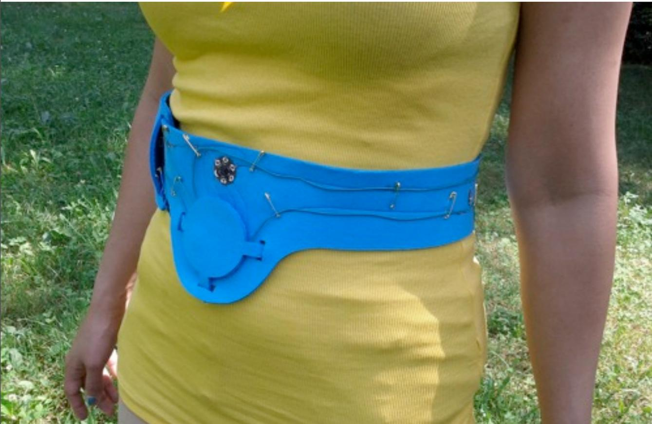
**The Balanceshirt made by laser cut acrylic felt, tilt sensors and lilypad to assist people with balance problems**
