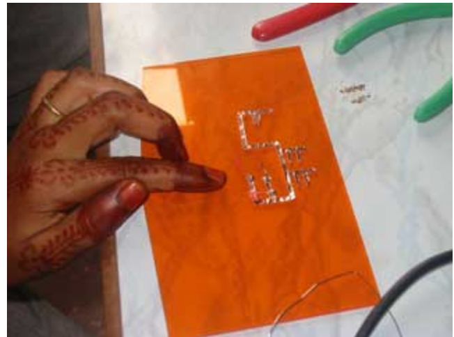
Figure 4: A printed circuit layout cut out of an adhesive copper sheet on the vinyl cutter and applied to a plastic board cut to size using the 3-D mill
