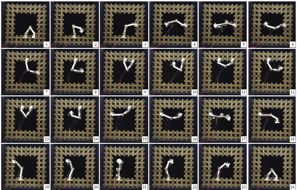
**Figure 15: Demonstration of climbing  $360^\circ$  around a loop using ankle rotation and upside down locomotion.** In steps 1-7, the robot uses ankle rotation to climb to the upper surface of the structure. In steps 8-13, the robot steps along the upper surface of the structure while hanging upside down. In steps 14-24, the robot uses two ankle rotation maneuvers to step to the side of the structure and then to return to its original position. Total elapsed time: 10 min.
