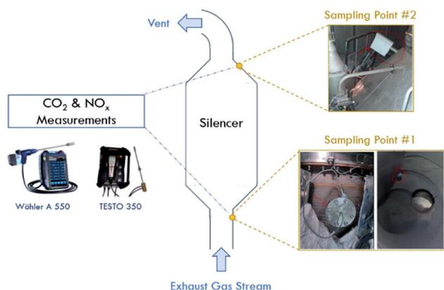
Fig. 1 Schematic diagram of the onboard emission monitoring system.
