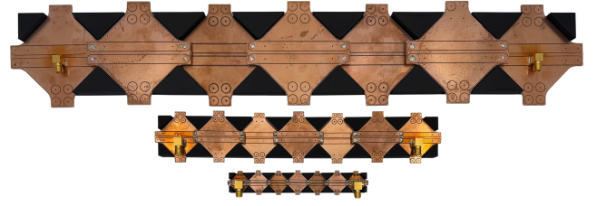
Fig. 13. Seven 64 mm-VMDs (top), seven 32 mm-VMDs (middle), and seven 16 mm-VMDs (bottom). VMDs with launches were de-embedded.
