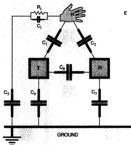
sensed,  $C_5$  is usually dominated by the capacitance through the shoes of the person. The ground terminal may either be a groundplane in close proximity to the transmitter and receiver, or the ambient room ground.
