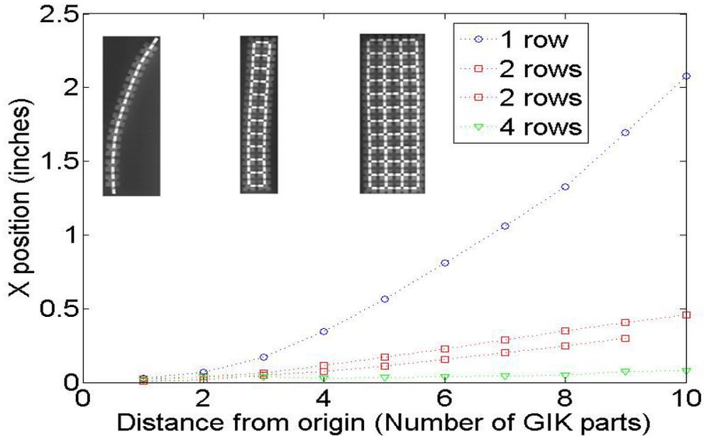
Figure 8: Experimental measurement of the error reduction as the size of the GIK structure increases from 1 row to 2 rows to 4 rows. 2 different measurement for the 2 row case was plotted to demonstrate the measurement precision.
