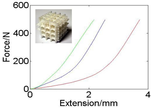
Figure 9: Isotropy tunability: different Young moduli in different directions.
