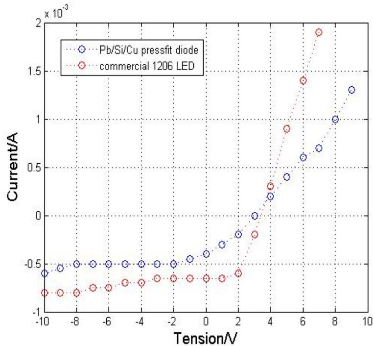
Figure 16: Current voltage characteristic for the GIK diode compared to a commercial Light Emitting Diode.
