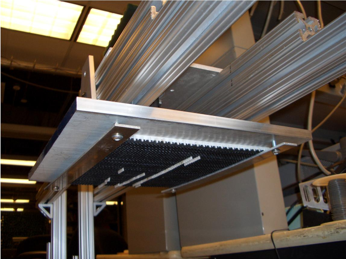
*Figure 30: Picture of the support plate to which is attached the GIK 1<sup>st</sup> layer. This first layer plays the role of the green plates for LEGO.*
