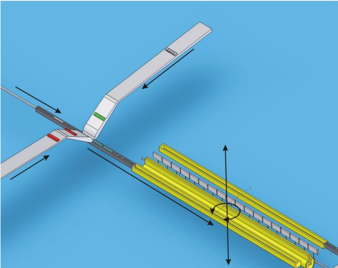
*Figure 22: The feeder is pushing in the building blade of the head the line to be added. A second feeder (not represented) is feeding the second building blade.*
