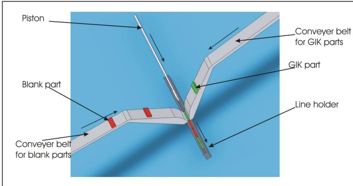
*Figure 25: Scheme of a feeder formed by 2 conveyor belts, one for vertical GIK one for Blanks. If more than 2 parts are needed more conveyor belts can be added. The parts are deposited in a line holder (dark gray) and a piston pushed the parts in the head when the line is built.*
