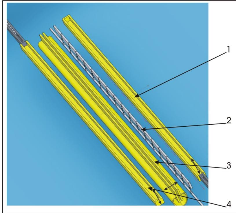
*Figure 23: The assembler head is composed of 4 blades. 1: building blade, 2: error detection blade, 3: line removing blade 4: line rebuilding blade. In construction mode the blades 3 and 4 only work if an error was detected. In disassembly mode, only blade 3 functions.*
