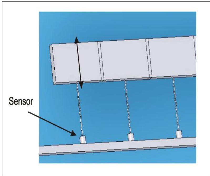
*Figure 24: The error detection blade is composed of a touch pad which is able to move up and down and a sensor which is sensing how much pressure is applied against each touch pad. An error is detected if there is a too high pressure difference between 2 adjacent pads.*
