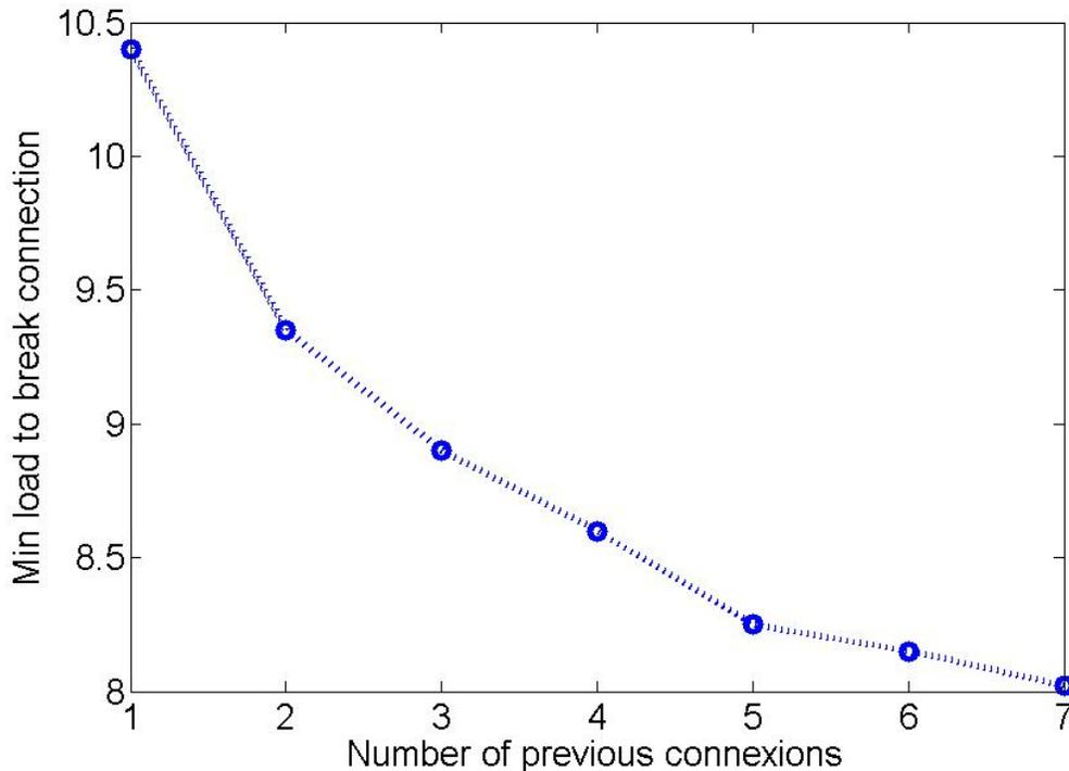
*Figure 26: Minimum load to break a connection as a function of the number of previous connections the 2 parts previously made. The more you connect two parts together and the easier it is to disconnect them. However the lower limit seems to be within 30% of the initial value which is acceptable.*
