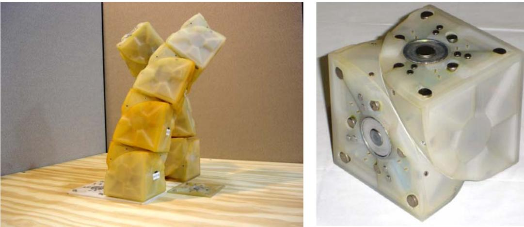
**Figure 8:** Zykov and Lipson's Molecubes swivel about their axis and use magnetic-latching to achieve self-reconfiguration. [30]
