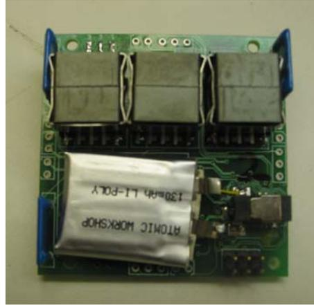
**Figure 53:** Driver board, top (**left**) and bottom (**lower**), showing 3 kV flyback power supplies, battery, microcontroller, and support circuitry.
