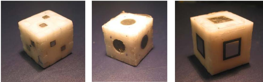
**Figure 39:** A few of the passive magnet-placement prototypes
