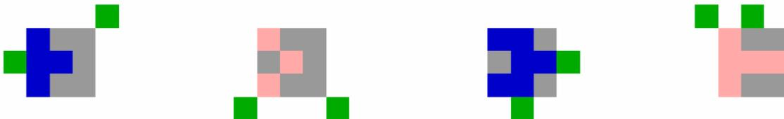
Figure 2-2: Logic CA gates (from left: AND, OR, XOR, NAND)
