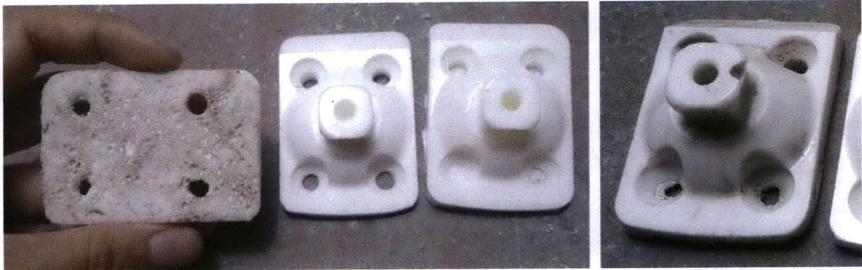
**Figure 7.26:** Casting a standard sized pyramid of Smooth-cast 300 polyurethane with kenaf reinforcements, Smooth-cast 300 polyurethane only, and Task 4 polyurethane. All casting resins from Smooth-on. On the right the top view of the kenaf-reinforced polyurethane.
