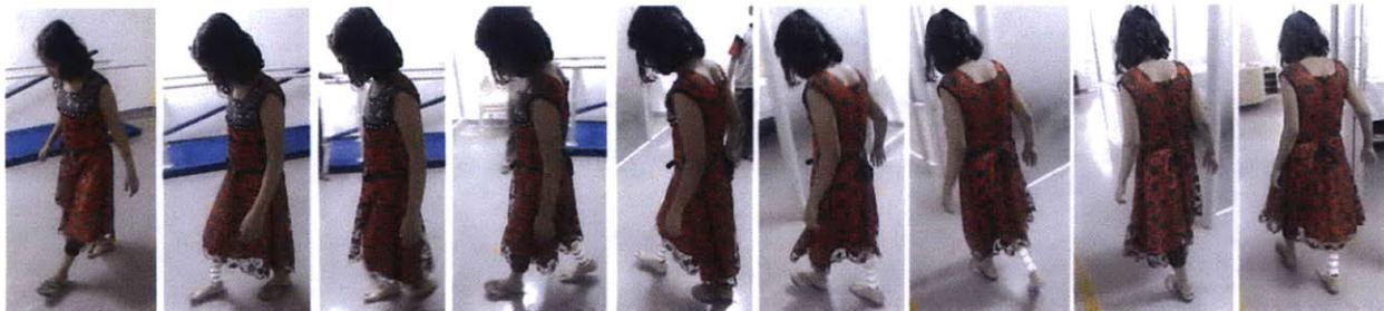
**Figure 7.36:** *The foot used in this test prosthesis is too large for the patient, making her gait poor during testing. She is unsure of her toe-off, and so looks at her feet as she is walking. The pylon makes some noises as some parts with play rub against each other, making her further uncertain of the prototype. As time went on, she became more comfortable, but still had awkward gait due to the wrongly sized foot.*
