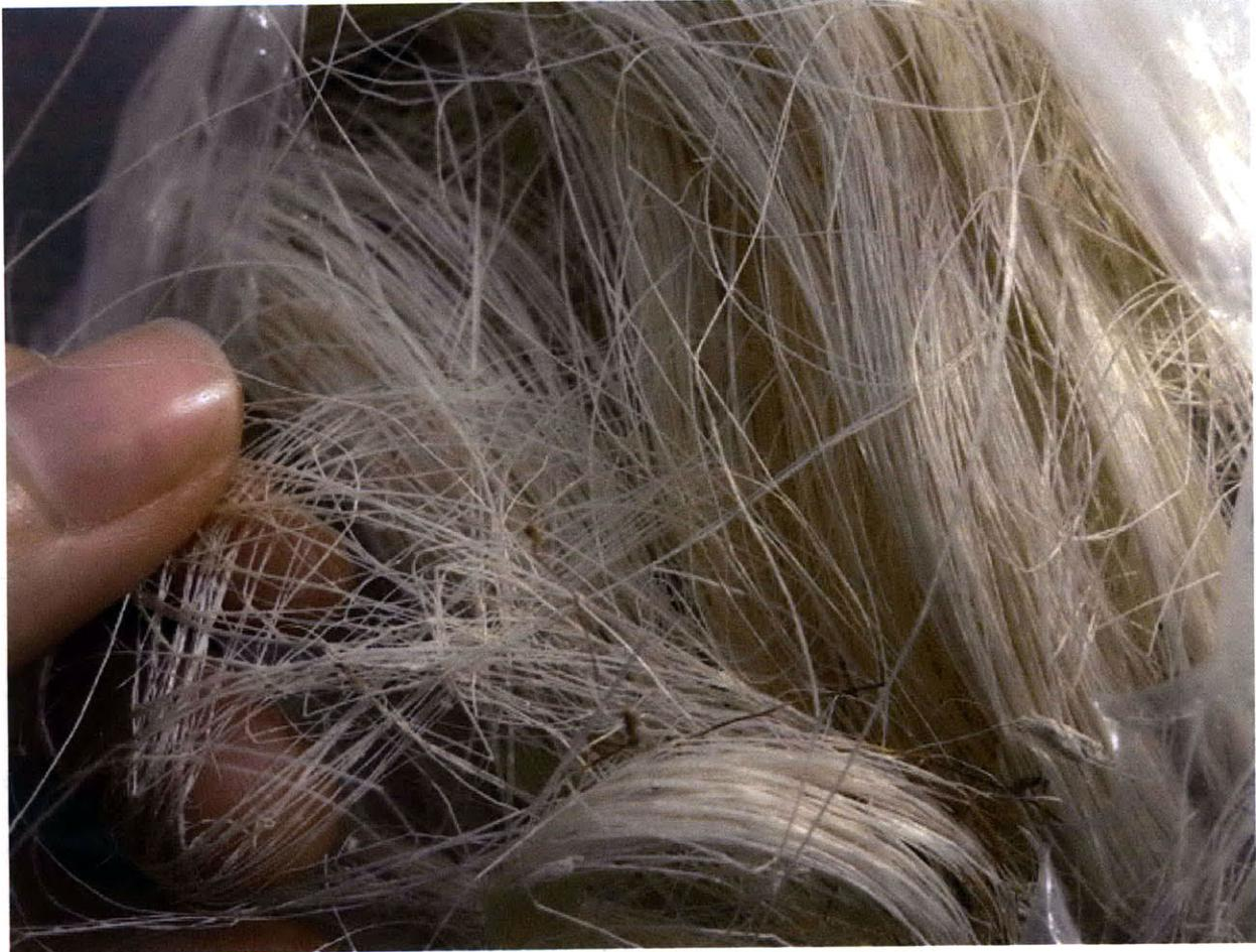
**Figure 3.2:** Decorticated sisal fibres from Reynolds Advanced Materials, Boston MA. Even within a single sisal fibre (which is a bundle of elementary fibres) there is a variation in width of up to 200%. The different part of the leaves produce different qualities of fibre, and this must be taken into account when producing parts with sisal.
