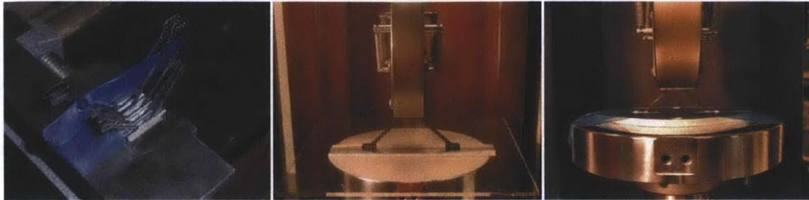
Figure 28 Initial Part Constraint Testing; Setup, Load Testing with Sliding Constraint, Load Testing with Fixed Constraint
