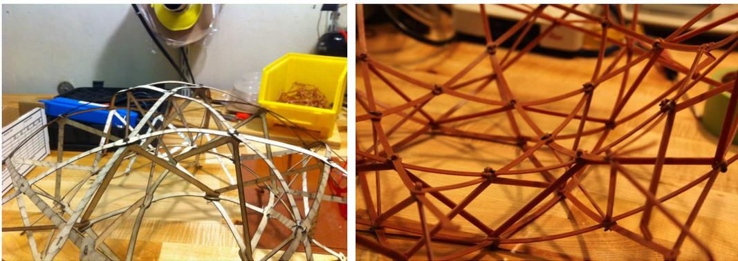
Figure 7.3: Sphere section prototypes from plywood and phenolic.
