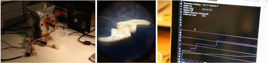
Figure 7.6: A) Ziploc extrusion machine, B) Microscope photograph of interlocking ziploc elements (roughly 6mm across), C) Graphical user interface for the extruder.
