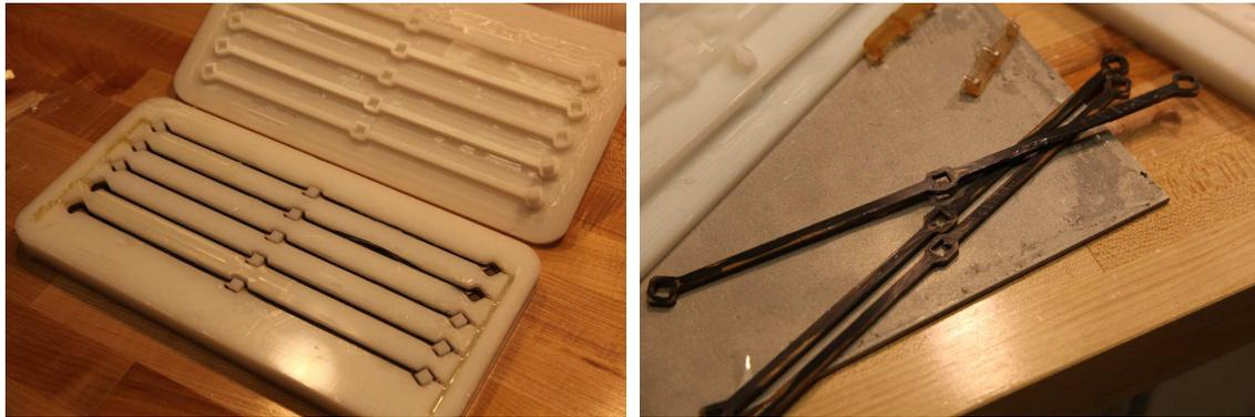
Figure 7.4: First vacuum balloon part prototyping
