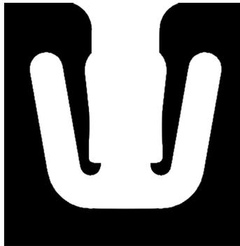
Figure 2-4: Potential scraping/wiping contact slot design.
