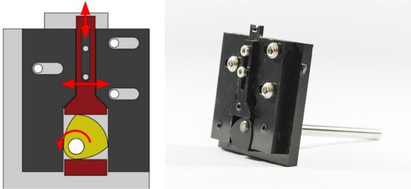
Figure 9-6: Rotary cam mechanism to produce discrete steps from continuous rotation.
