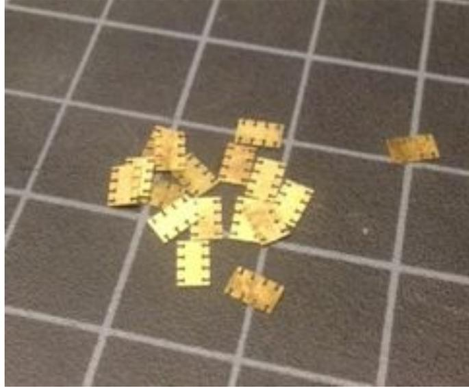
Figure 2-10: Brass parts milled on the Hurco
