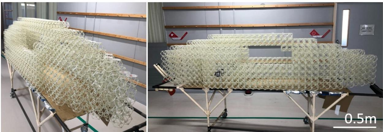
Figure 4-10: Completed lattice car frame.
