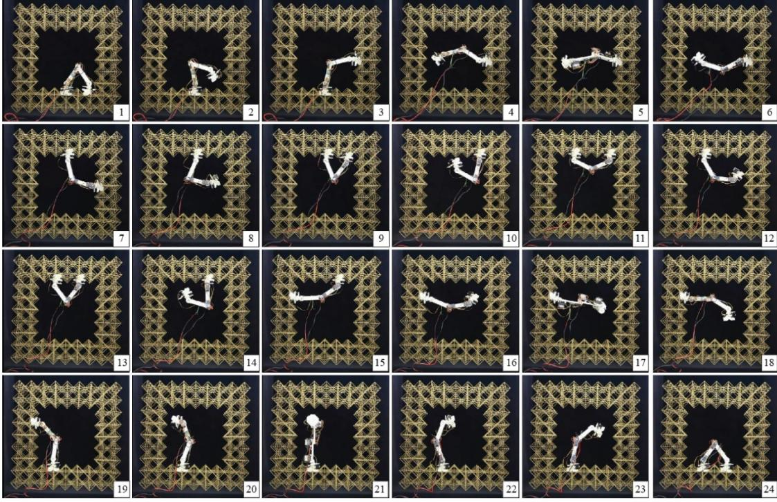
Figure 3-11: Demonstration of climbing  $360^\circ$  around a loop. (1-3) Concave cornering, (4-6)  $180^\circ$  ankle rotation, (7-9) concave cornering, (10-12) stepping, (13-15) concave cornering, (16-18)  $180^\circ$  ankle rotation, (19-20) concave cornering, (21-24)  $180^\circ$  ankle rotation, end sequence. Total elapsed time: 10 min. From [100]
