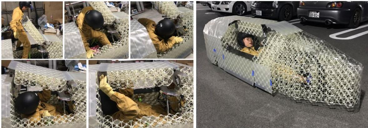
Figure 4-15: Driver entrance and preliminary vehicle testing.
