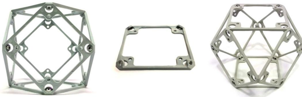
Figure 2-21: Rigid lattice. (Top) Built 4x4x4 voxel cube, (bottom) single voxel and face part.
