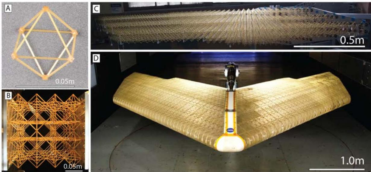
Figure 4-20: MADCATv1 [21]. (A) Modular building block unit, (B) 4x4x4 unit cube during mechanical testing, (C) Single half-span wing structure composed of 2088 building block units, (D) Blended wing body aerostructure with skin, mounted to central load balance in the 14x22 subsonic wind tunnel at NASA Langley Research Center.
