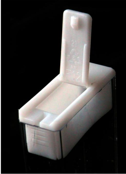
(a) The injection molded plastic lid from a Tic-Tac candy dispenser, showing an integrated flexural hinge [66].
