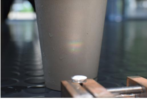
(a) Ruled grating splitting sunlight into a rainbow, which is projected onto a cup.
