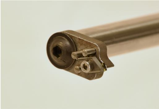
(a) Grating ruling tool, initially a sharp carbide insert, later the piece of CVD diamond scrap shown here.
