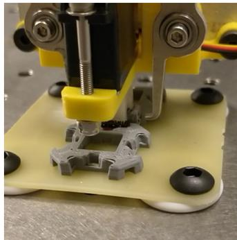
(e) Picking up a strut; notice milled Delrin placement foot.
