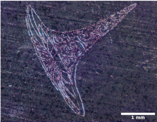
(a) Close-up image of engraved black hole, showing good detail but some evidence of work shifting during the operation.
