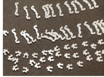
(c) A collection of machined Delrin clips for Meso-DICE struts and nodes.
