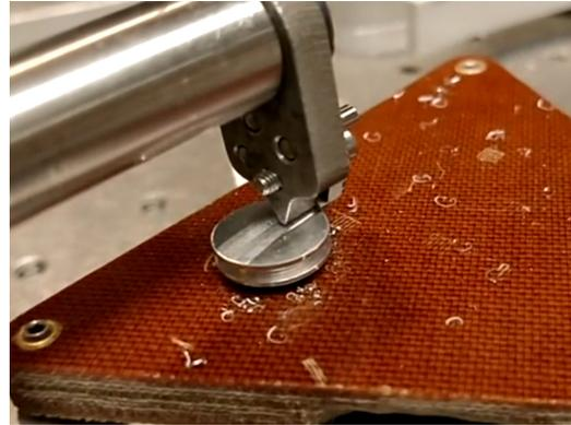
(b) Freeze-frame from grating ruling video showing tool scratching fine grooves into an aluminum SEM sample holder.
