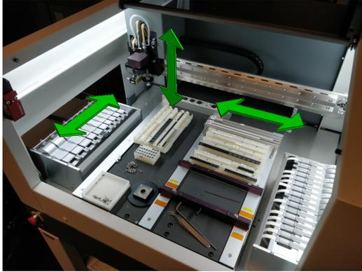
(a) Mechatronika M20V pick-and-place machine, used for electronics assembly.
