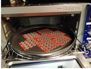
(b) Removing 112 Meso-DICE strut PCBs from the reflow oven.
