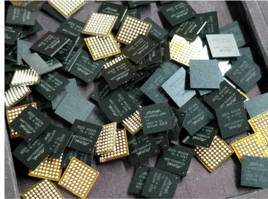
(b) A pile of uninstalled 3x3 mm WLCSP ATSAMD51J20s randomly oriented to show 0.4 mm spaced solder ball contacts.
