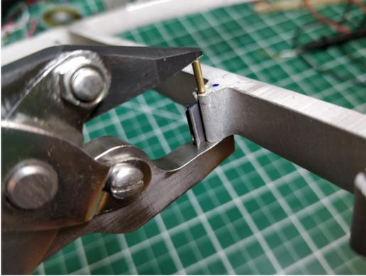
(a) Pinsetter tool made by fabricating a custom lower jaw for a pair of common parallel-jaw pliers.
