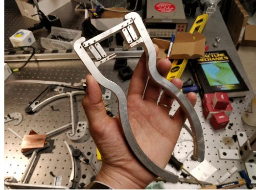
(b) Recursive pinsetter made with ten modular superelastic flexures and an aluminum frame.
