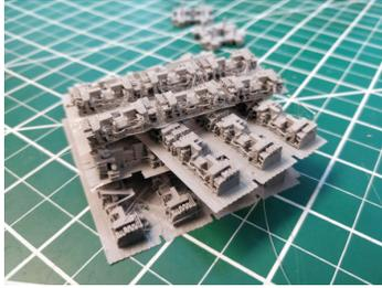
(d) 3D printed alignment pieces before removing support material.
