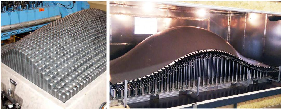
Figure 1-1: A) A 2688 actuator  $1 \times 1.8m$  reconfigurable die for sheet metal forming built by David Hardt at MIT [36]. B) Reconfigurable composite layup die using NEMA packaged steppers and leadscrews [2].
