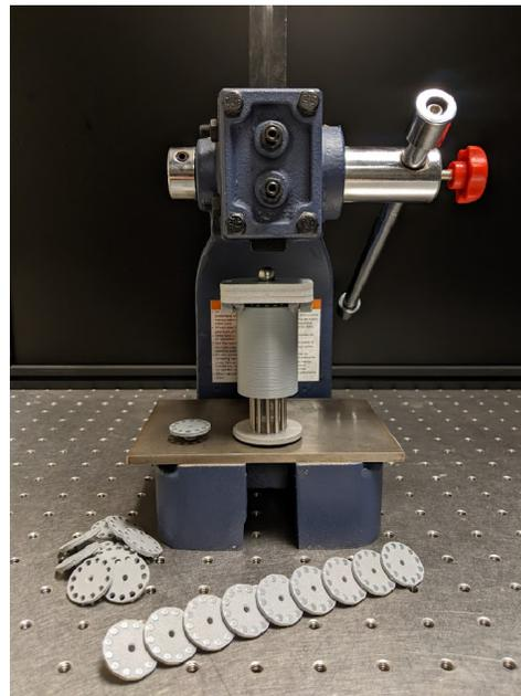
Figure 2-9: Rotor stamping jig and section view
