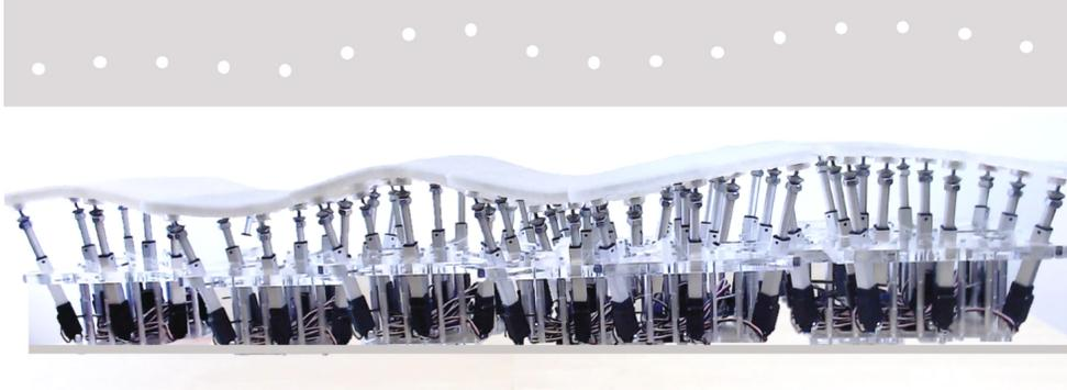
Figure 1-3: An interpolated shape display intended for augmented and virtual reality [47].
